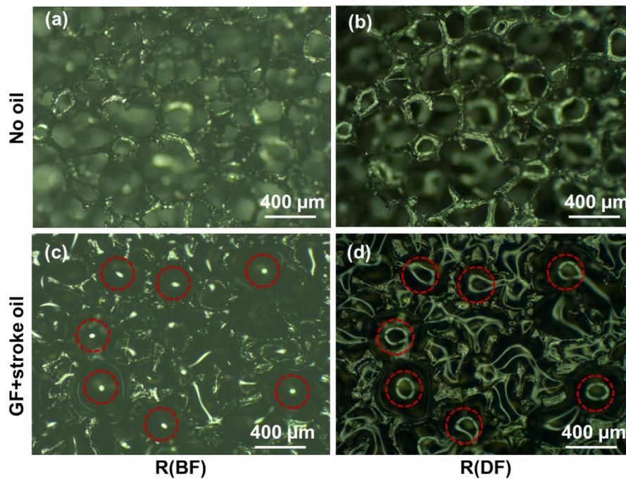
**S2. Optical images with reflected light of graphene foam (a) , (b) without and (c),(d) with stroke oil. (a) and (c) are under bright field while (b) and (d) are under dark field.**
