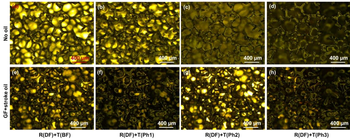
**S5. Optical images with both reflected (dark field) and transmitted light of graphene foam (a)-(d) without and (e)-(h) with stroke oil. Four modes are shown, with each column is at the same detection mode.**
