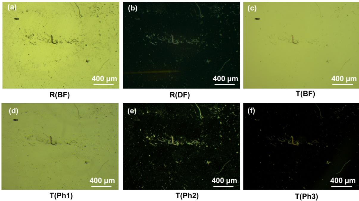
**S1. Images of glass slide with some stains under different detection modes of Zeiss A1 microscope. (a) Bright field and (b) Dark field modes for reflected light; (c) Bright field and (d)-(f) Phase contrast modes for transmitted light. Ph 1, Ph 2 and Ph 3 represent for different ring diaphragm, which can achieve various medium numeral apertures.**
