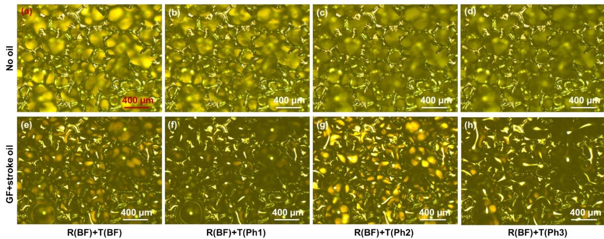
**S4.** Optical images under reflected (bright field) and transmitted light of graphene foam (a)-(d) without and (e)-(h) with stroke oil. Images in the same column are at the same detection mode.
