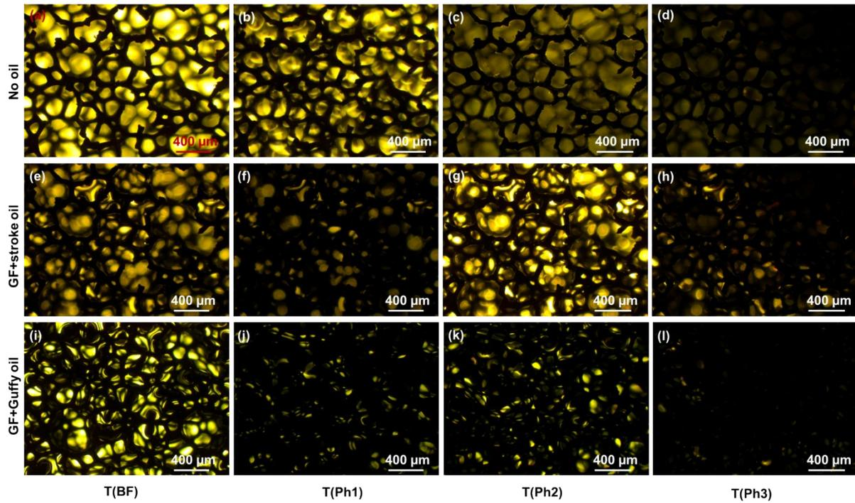
**S3.** Optical images with only transmitted light of graphene foam (a)-(d) without , (e)-(h) with stroke oil and (i)-(l) with Guffy field oil . Images in the same column are at the same detection mode, with (a) bright field and (c)-(d) phase contrast modes.
