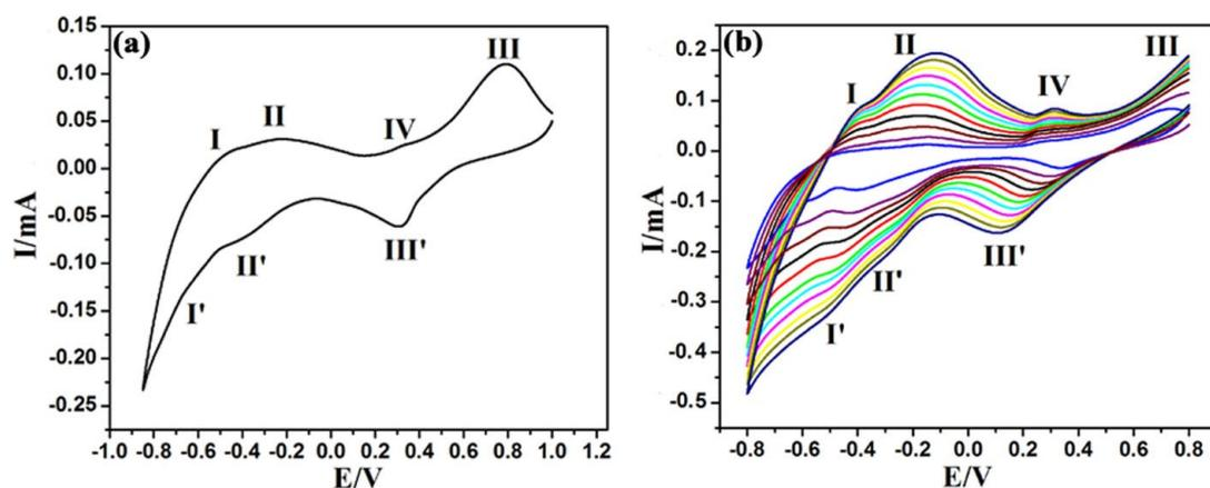
**Figure S9** (a) Cyclic voltammograms of **1-CPE** in 1 M H<sub>2</sub>SO<sub>4</sub> aqueous solution. Potentials vs.SCE. Scan rate: 20mVs<sup>-1</sup>. (b) Cyclic voltammograms of **1-CPE** in 1M H<sub>2</sub>SO<sub>4</sub> solution at different scan rates (from inner to outer:20,50,80,110,140,170,200,230,260,290,320mV.s<sup>-1</sup>).
