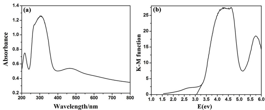
**Figure S6** (a) Solid state UV-vis spectra and, (b) the diffuse reflectance spectra of compound **1**.
