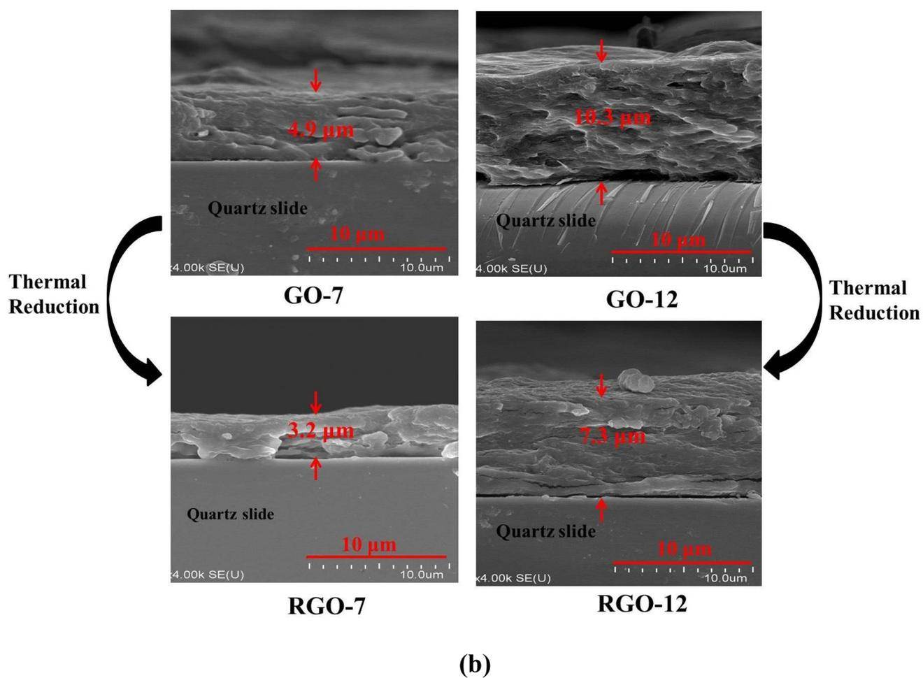
Fig. S4: (a) Schematic illustration of barrier effect of GO or RGO filled LbL coating; (b) SEM images of the fractured surfaces of GO coated multilayer films on quartz slide before (GO-7 and GO-12) and after (RGO-7 and RGO-12) thermal reduction.
