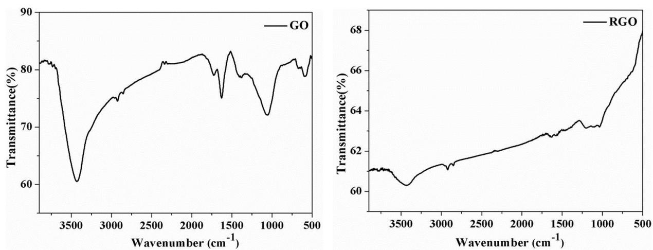
Fig. S5 FTIR spectra of GO and RGO.
