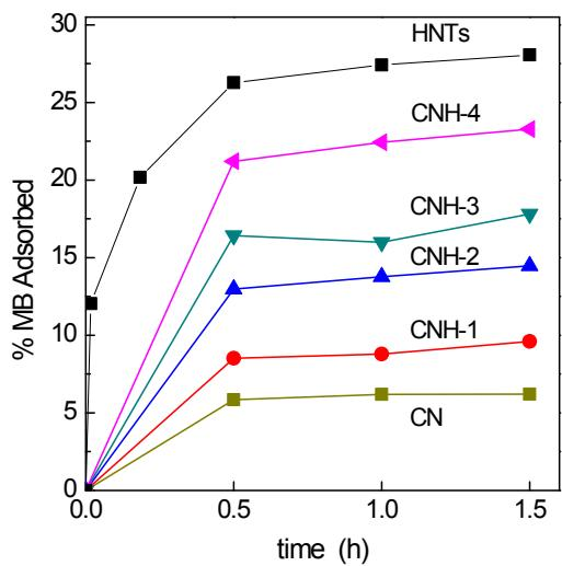
**Figure S8.** MB adsorption on the pure  $\text{g-C}_3\text{N}_4$ , HNTs and CNH- $x$  photocatalysts in the dark. For the  $\text{g-C}_3\text{N}_4$  and CNH- $x$  nanocomposites,  $1.25 \text{ g L}^{-1}$  of the material was used. For the HNTs,  $0.125 \text{ g L}^{-1}$  were used, e.g. equal amount of HNTs in the CNH-4 sample.
