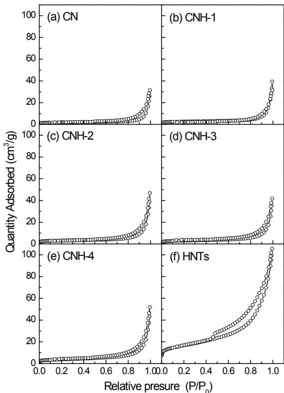
**Figure S3.** Nitrogen adsorption-desorption isotherms of  $\text{g-C}_3\text{N}_4$  (a), HNTs (f) and the HNTs/ $\text{g-C}_3\text{N}_4$  ((b)-(e)) nanocomposites.
