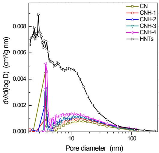
**Figure S4.** Pore size distribution of the samples calculated from the desorption branch of the  $\text{N}_2$  isotherm using the BJH method.
