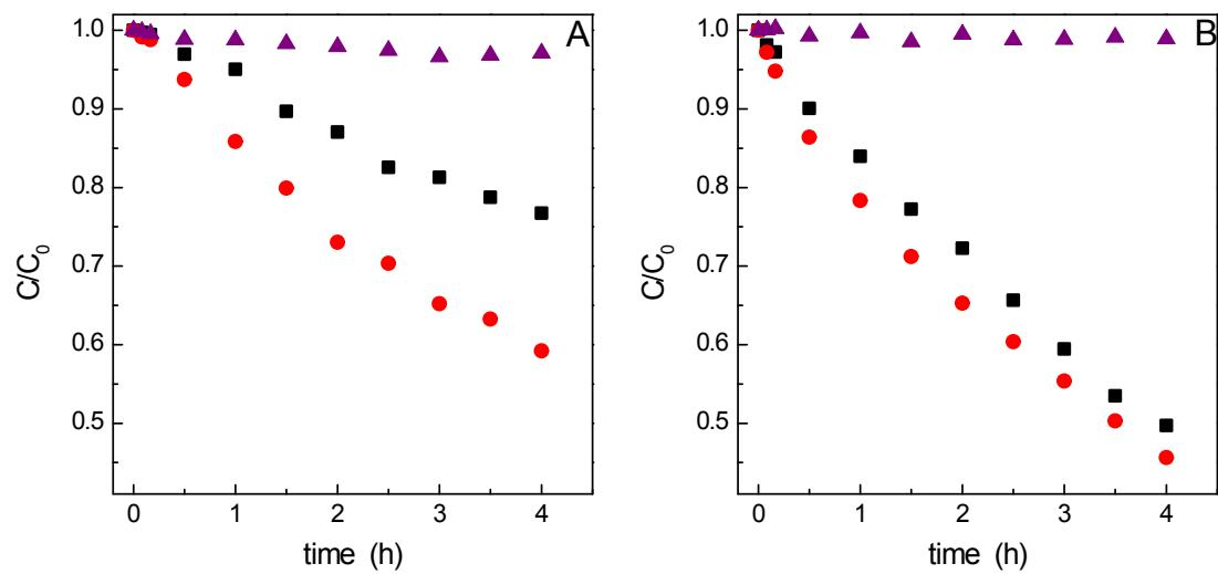
**Figure S10.** Photocatalytic degradation of phenol (A) and MO (B) over the pure  $\text{g-}\text{C}_3\text{N}_4$  (black), HNTs (purple) and CNH-2 (red) photocatalysts under simulated solar light irradiation.
