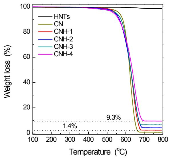
**Fig. S5.** TGA profiles of the g-C<sub>3</sub>N<sub>4</sub>, HNTs and of the as-prepared HNTs/g-C<sub>3</sub>N<sub>4</sub> nanocomposites.
