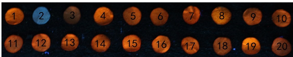
Fig. S10. Color changes of test paper with different species. 1: probe 1 alone; 2–20: probe 1 + \text{HSO}_3^- , \text{HS}^- , \text{F}^- , \text{Cl}^- , \text{Br}^- , \text{I}^- , \text{AcO}^- , \text{ClO}_4^- , \text{NO}_3^- , \text{N}_3^- , \text{SO}_4^{2-} , \text{HSO}_4^- , \text{SCN}^- , \text{PO}_4^{3-} , \text{HPO}_4^{2-} , \text{H}_2\text{PO}_4^- , Cys, Hcy and GSH.
