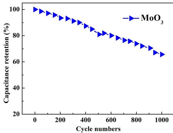
**Fig. S1** Cycle stability of MoO<sub>3</sub> at a current density of 1A·g<sup>-1</sup> in 1M KOH solution.
