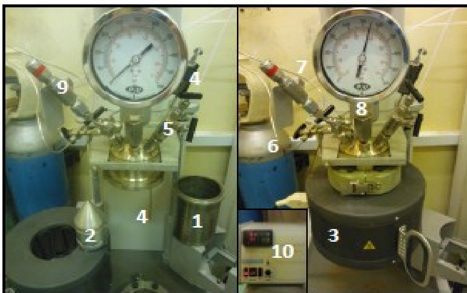
Fig. S7 Snapshots of autoclave (Parr mod. 4523 Bench Top Reactor, 1L capacity) adapted for batch-mode CO 2 absorption into MgO/Mg(OH) 2 promoted by saturated steam: 1. Reactor pot; 2. Sample holder; 3. Oven (with 5 thermocouple); 4. Temperature gauge; 5. Discharge valve (vent); 6. CO 2 feed; 7. N 2 feed; 8. Pressure gauge; 9. Safety release valve (50 bar); 10. Temperature controller.
