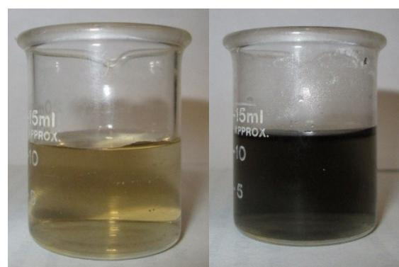
Fig. S7. (Left) As-prepared GO solution diluted 10 times in water. (Right) Reduced GO (rGO) obtained after the addition of 2 mL of 0.1 mol L<sup>-1</sup> ascorbic acid and heating at 70 °C for 12 hours.
