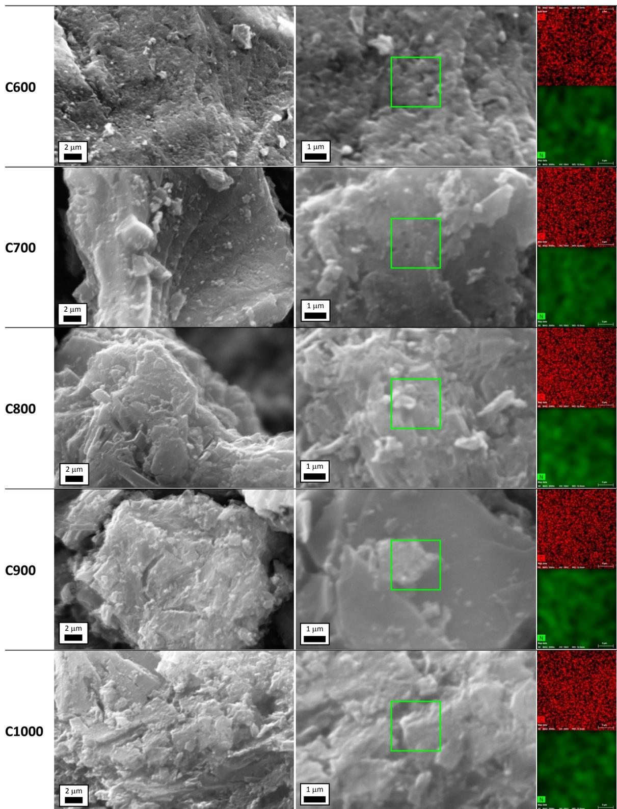
Figure S5. Scanning electron micrographs of carbons C600–C1000, and energy dispersive X-ray spectroscopy (EDS) maps of carbon (red) and nitrogen (dark green) in the areas marked by a green square.
