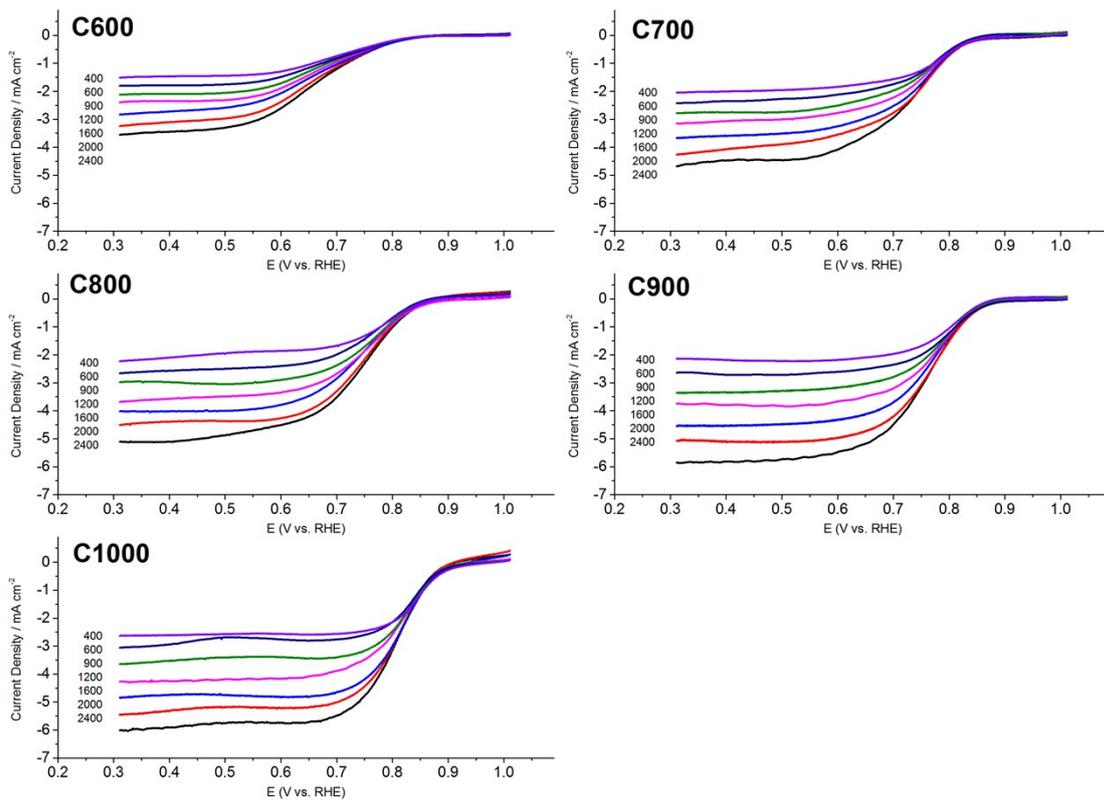
Figure S6. Rotating disk electrode LSVs of ORR electrocatalysis in 0.1 M KOH along the carbon series, at different rotation speeds in rpm, 10 mV/s.
