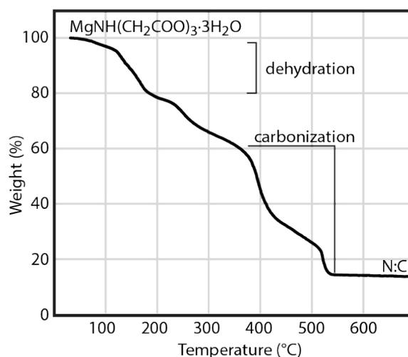
Figure S1. Thermal gravimetric analysis of MgNTA in argon, heating rate 20 °C/min. Identical results were obtained at a slower heating rate(10 °C/min).
