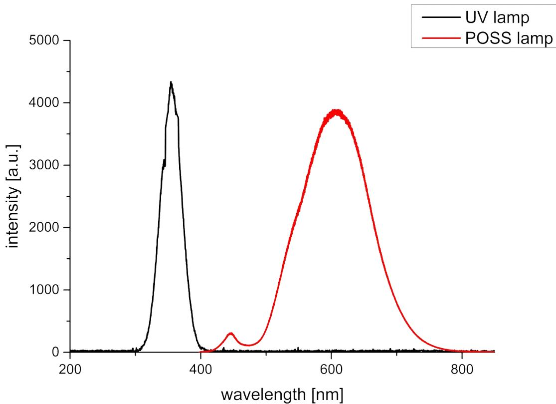
**Figure S2.** Intensity spectra of longwave UVA irradiation provided by the UV lamp (Waldmann Typ 602352 lamp, 230V, 50Hz, 2x4W) and of the LED lamp (R11/D3/N/B, Relco Group Ltd, 3W) of the portable oxidative stress sensor used in the experiments. At a wavelength of 350 nm the power of the UV lamp at the sample was  $60 \mu\text{W cm}^{-2}$ . The power of the LED diodes at the sample was  $25 \text{ mW cm}^{-2}$  at a wavelength of 550 nm.
