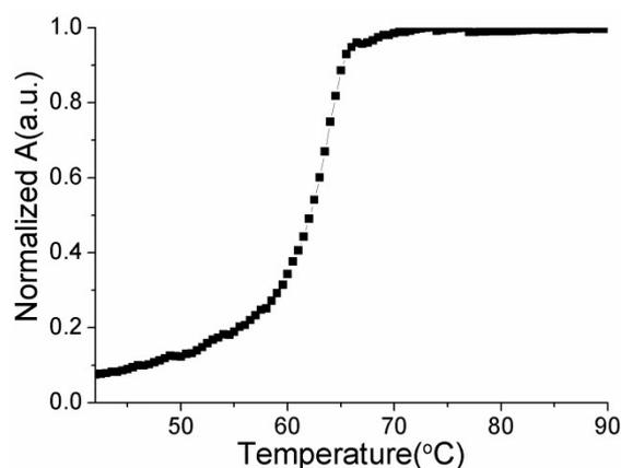
**Fig. S2**  $T_m$  measurements of DNA dendrimer ( $G_4$ )
