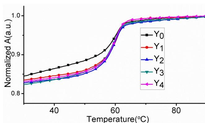
**Fig. S1**  $T_m$  measurements of Y-DNA. UV melting experiments were carried out by monitoring the absorbance at 260 nm. The concentration of Y-DNA was 1.3  $\mu\text{M}$  each.
