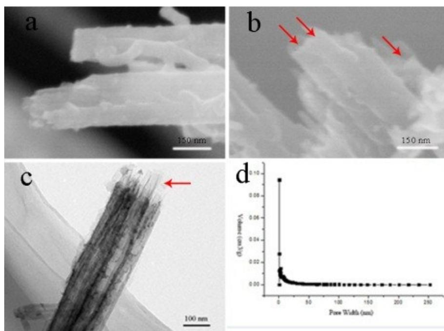
Fig. S1 (a-b) the cross sectional SEM images of MoS<sub>2</sub>/VACNTs-2, (c) TEM image of MoS<sub>2</sub>/VACNTs-2, (d) pore size distribution curves of VACNTs
