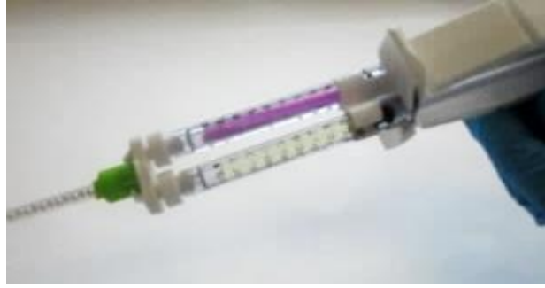
Fig. S9 Possible double syringe application of the Au-(PEG) 4 -BAG10 nanocomposite hydrogel.
