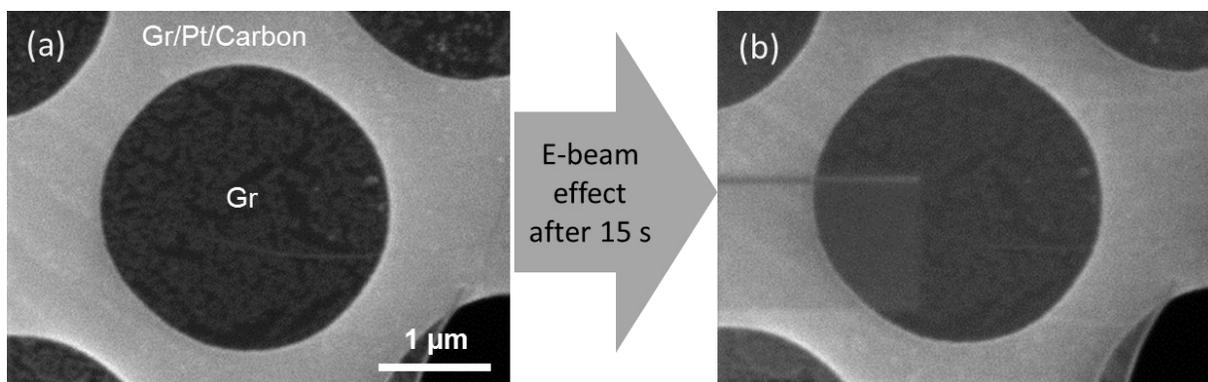
**Figure S6.** E-beam induced carbon contamination of a graphene membrane transferred by PMMA onto a carbon mesh with Pt and annealed on a hot plate.
