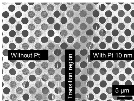
**Figure S5. Spillover of Pt catalysis.** SEM image of suspended graphene transferred by PMMA on a carbon mesh with a pre-deposited 10 nm Pt layer (right side) and without Pt (left side). Both the region with and without Pt are separated by a transition section (in the center) which is not covered by Pt, but represents graphene membranes cleaned by hydrogen diffused here from the Pt area.
