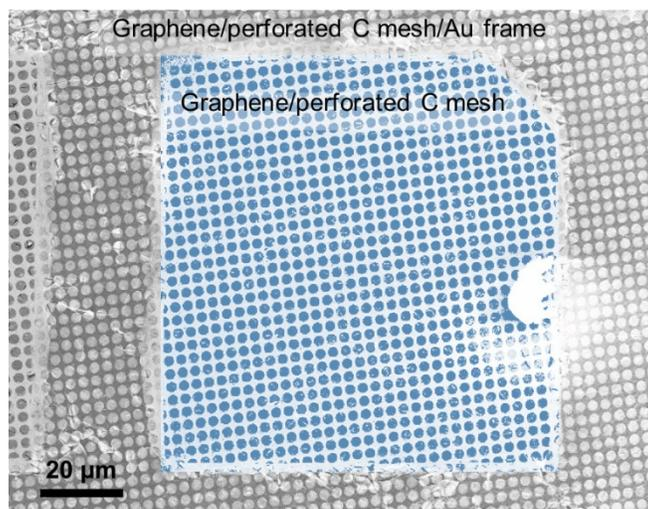
**Figure S3. SEM image showing perforated carbon mesh covered with as transferred suspended graphene (false blue color) Surface coverage ( $\approx 95\%$  before anthracene cleaning procedures) was calculated as the ratio of orifices covered with graphene to all orifices in carbon mesh.**
