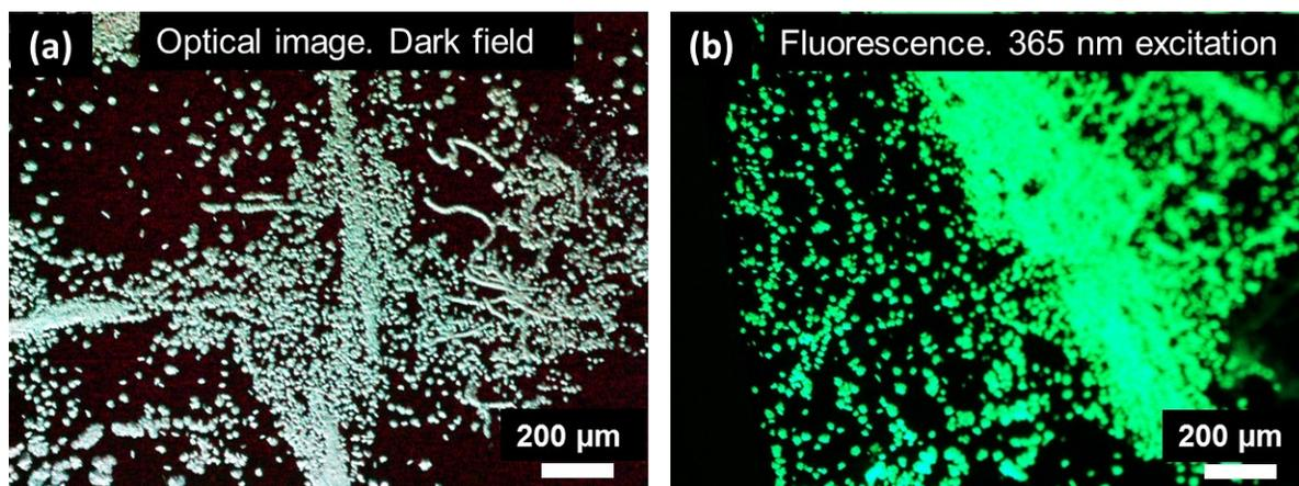
**Figure S2. The morphology of the anthracene film deposited onto Gr/copper stack held at the room temperature.** (a) Dark field optical image. The dark areas correspond to pristine graphene on copper. (b) Fluorescent microscopy image of the same region as in (a) excited by 365 nm UV light.
