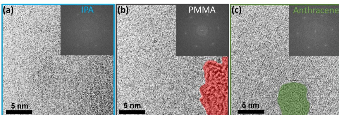
**Figure S7.** HRTEM images and fast Fourier transforms (FFTs) (insets) of graphene transferred by IPA (a), PMMA (b), and anthracene (c) onto a carbon mesh with Pt catalyst. Color coded regions have been excluded from FFT analysis.
