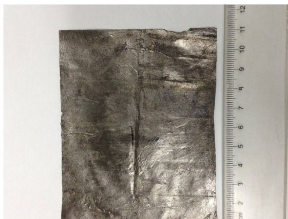
5 Figure S5. Electrochemical reduction preparation of rGO film covered on an irregular lens paper.
