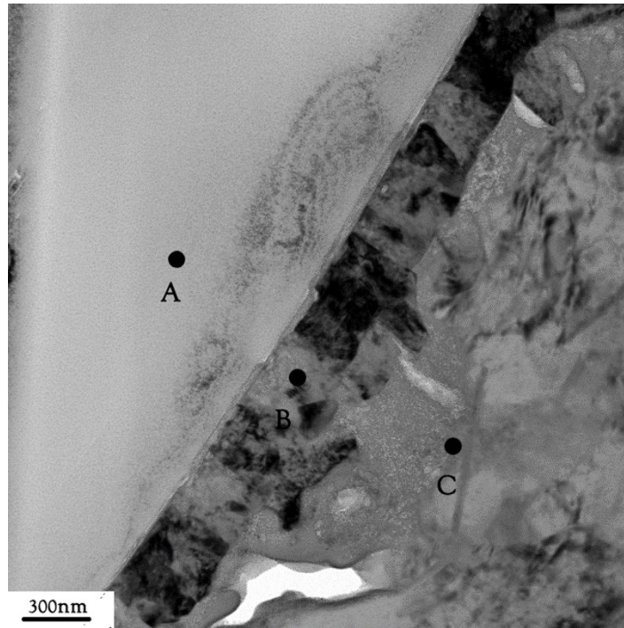
Fig. S2. An overview TEM bright-field (BF) image of the Si-coated G_f /Cu interface
