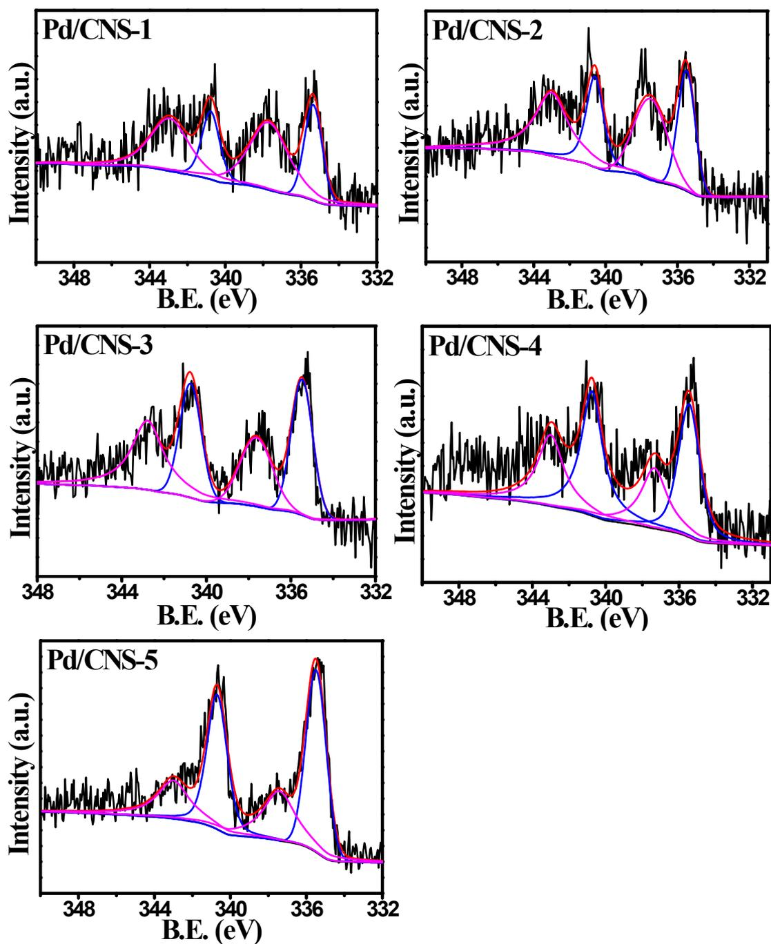
Fig. S6 The Pd 3d high-resolution XPS spectra of Pd/CNS-1, Pd/CNS-2, Pd/CNS-3, Pd/CNS-4, and Pd/CNS-5 catalysts.
