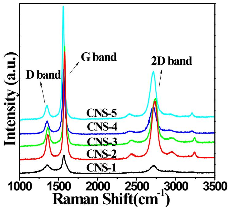
**Fig. S2** Raman spectra of CNS-1, CNS-2, CNS-3, CNS-4 and CNS-5 supports
