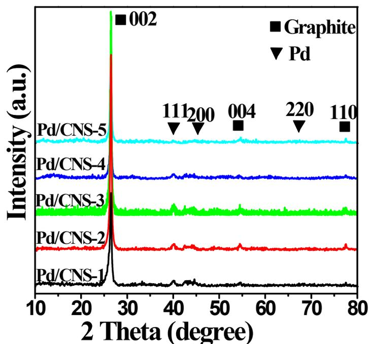
**Fig. S5** XRD patterns of Pd/CNS-1, Pd/CNS-2, Pd/CNS-3, Pd/CNS-4 and Pd/CNS-5 catalysts.
