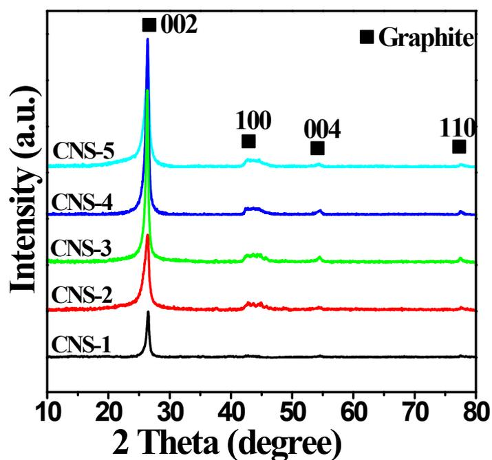
Fig. S1 XRD patterns of CNS-1, CNS-2, CNS-3, CNS-4 and CNS-5 supports
