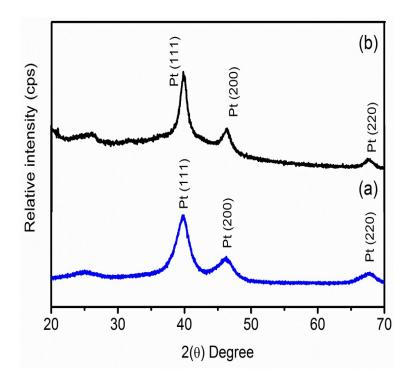
**Fig. 3S.** X-ray diffraction pattern of Pt deposited on carbon (a) before ADT and (b) after 80 h of ADT.
