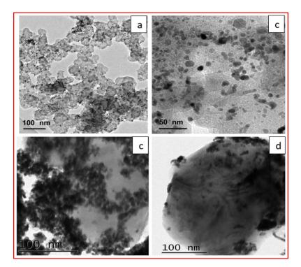
**Fig. 5S.** HR-TEM image of Pt/C and Pt/TiON-Co cathode electrocatalyst (a & b) before ADT, (c & d) after 80 h of ADT.
