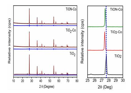
**Fig. 1S.** XRD refinement for  $TiO_2$ ,  $TiO_2$ -Co and TiON-Co and their major plane (110) peak shift.
