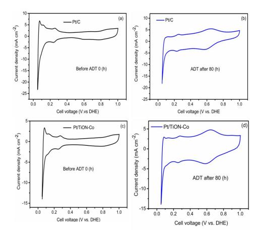
**Fig. 2S.** PEFCs with CV at room temperature with scan rate of 50 mV s<sup>-1</sup>. (a) Pt/C before ADT (b) Pt/C after 80 h of ADT and (c) Pt/TiON-Co before ADT and (d) Pt/TiON-Co after 80 h of ADT.
