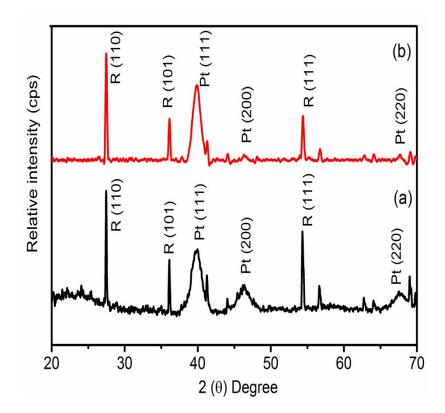
**Fig. 4S.** X-ray diffraction pattern of Pt deposited on TiON-Co electrocatalyst (a) before ADT and (b) after 80 h of ADT.
