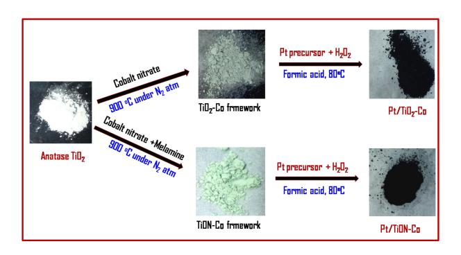
**Scheme 1:** Various stages of colour change are observed for preparation of Pt deposited on TiO<sub>2</sub> electrocatalysts.
