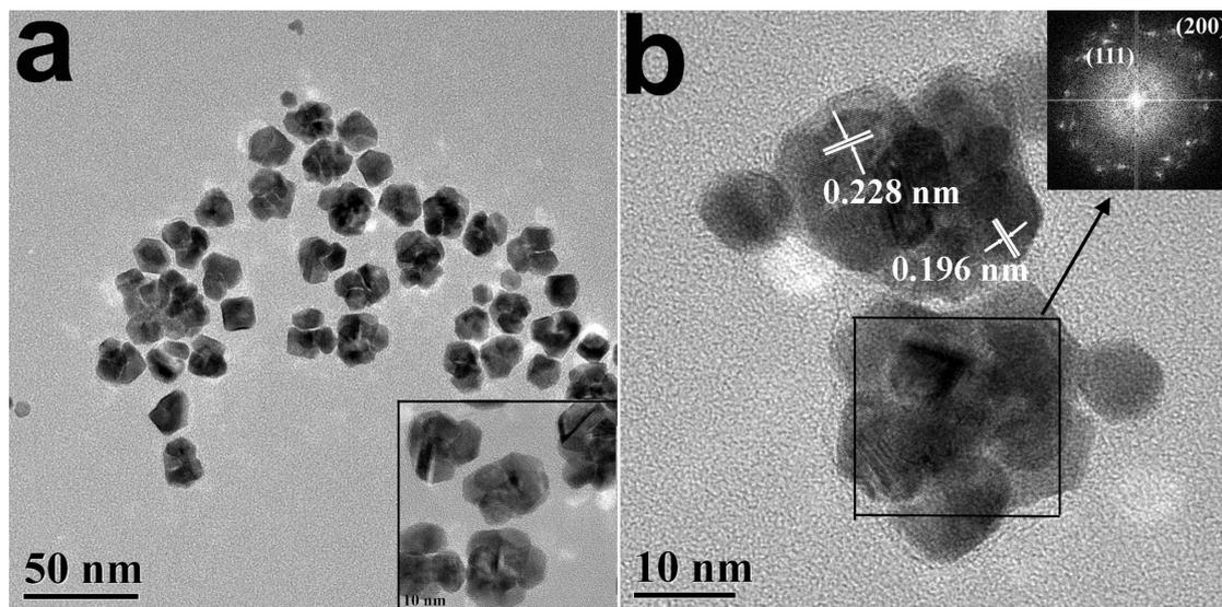
**Fig. S2** TEM image (a), HRTEM images (b), and corresponding FFT image (inset of b) of as-obtained Pt multipolyhedral nanostructures in typical synthesis with the mixture of ethylene glycol and water as solution.
