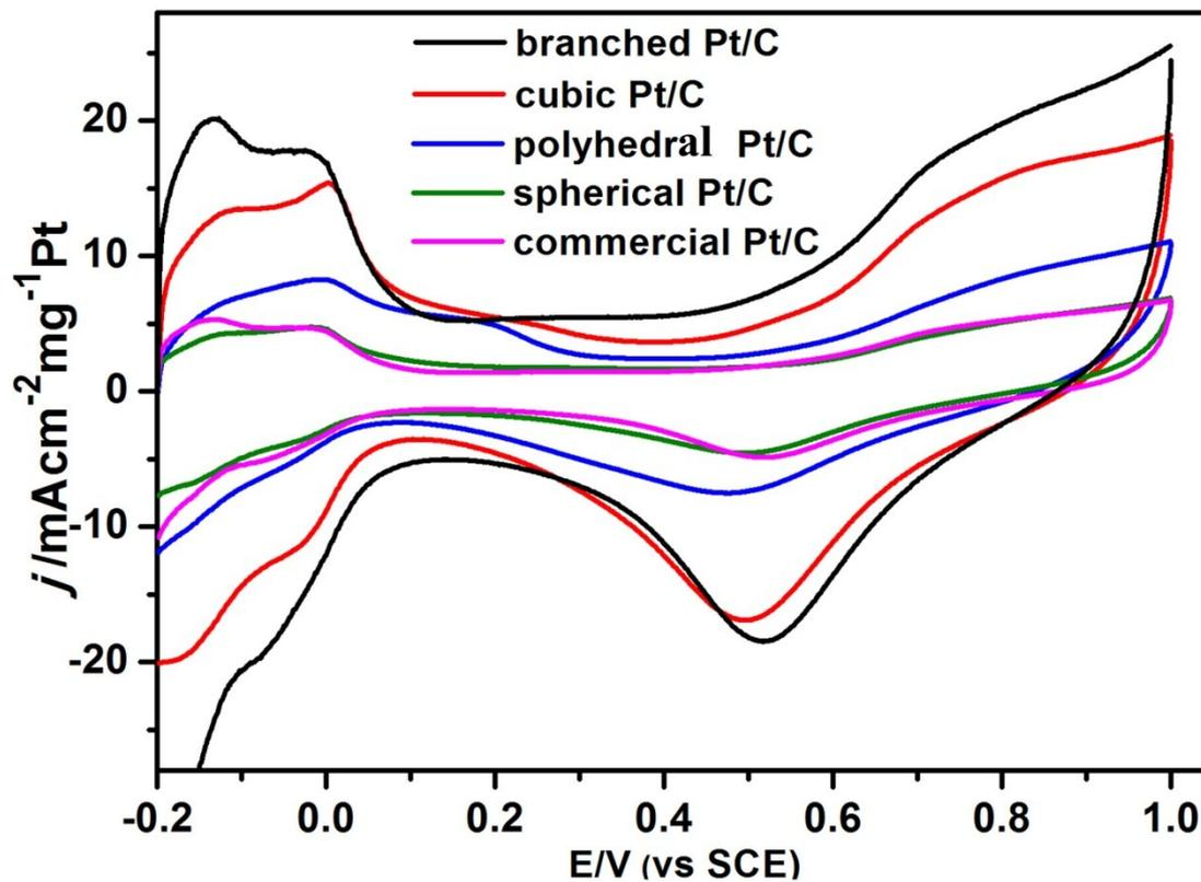
**Fig.S5** Cyclic voltammetric curves of Vulcan XR-72 loaded with as-obtained four different shaped Pt nanocrystals and commercial Pt nanoparticles in 0.5 M  $\text{H}_2\text{SO}_4$  with a sweep rate of  $50 \text{ mV}\cdot\text{s}^{-1}$ .
