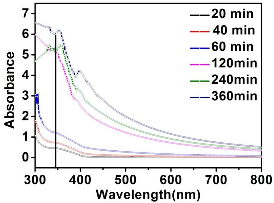
**Fig. S1** UV-vis spectra of the time evolution of substrate concentration for as-obtained polyhedral nanocrystals in typical synthesis with glycerol-water as solution.
