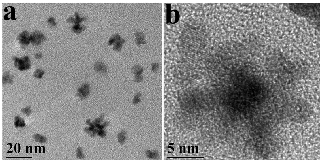
**Fig. S4** TEM image (a) and HRTEM images (b) of as-obtained Pt nanostructures in typical synthesis (glycerol-chloroform mixture) with temperature of 200°C.
