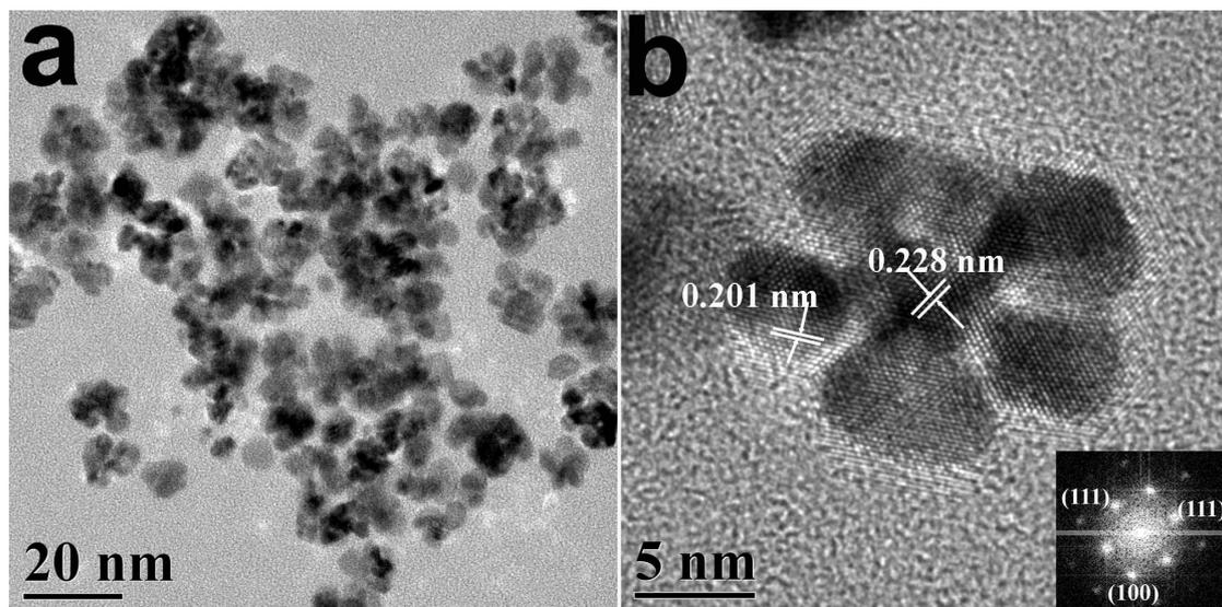
**Fig. S3** TEM image (a), HRTEM images (b), and corresponding FFT image (inset of b) of as-obtained flower-like Pt nanostructures in typical synthesis (glycerol-water mixture) with oxalic acid substitution for benzoic acid.
