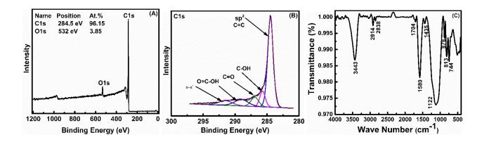
Fig 1S: Characterization of as-synthesized CNO (A) wide scan XPS spectrum, (B) C1s spectrum and (C) FT-IR spectra, showing the presence of oxygen functionalities.
