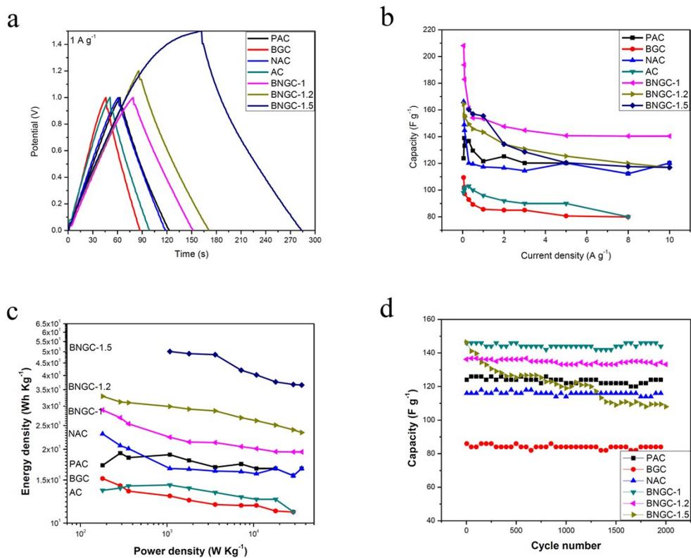
Fig.s2 (a) GCD curves of all the samples and BNGC at different potential windows; (b) the specific capacitance of all the samples at different current density; (c) Ragone plots referring to energy and power density of the prepared carbons; (d) cycle life of the prepared carbon materials at current density of 1 A/g.
