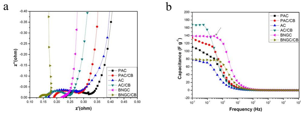
Fig.s3 the Nyquist plot (a) and the capacitance-frequency plot (b) for the influence of CB.
