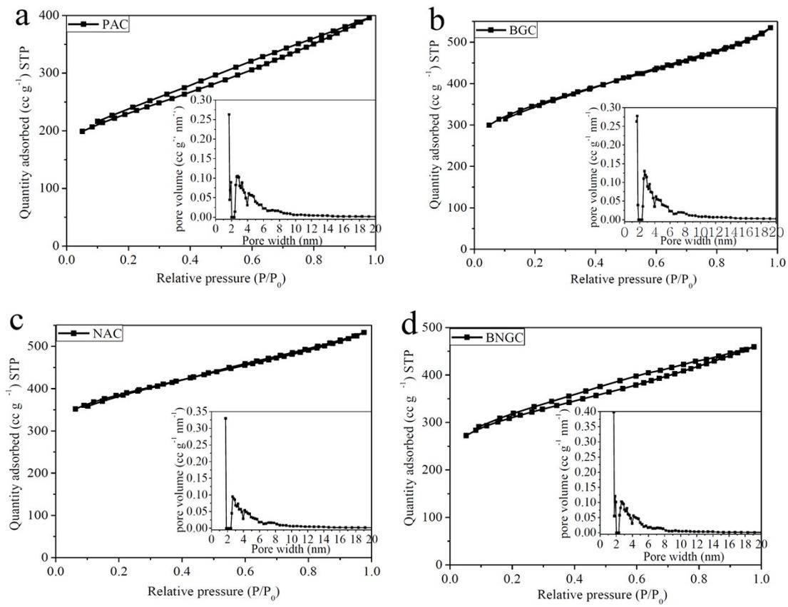
Fig.s1 Nitrogen adsorption/desorption isotherms of sample (a) PAC, (b) BGC, (c) NAC and (d) BNGC.
