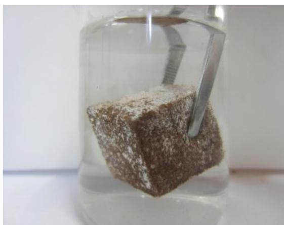
**Fig. S7.** Mirror-like phenomenon can be observed on the LMF sponge in the water after 1000 cycles of compression testing at the strain value of 60%.
