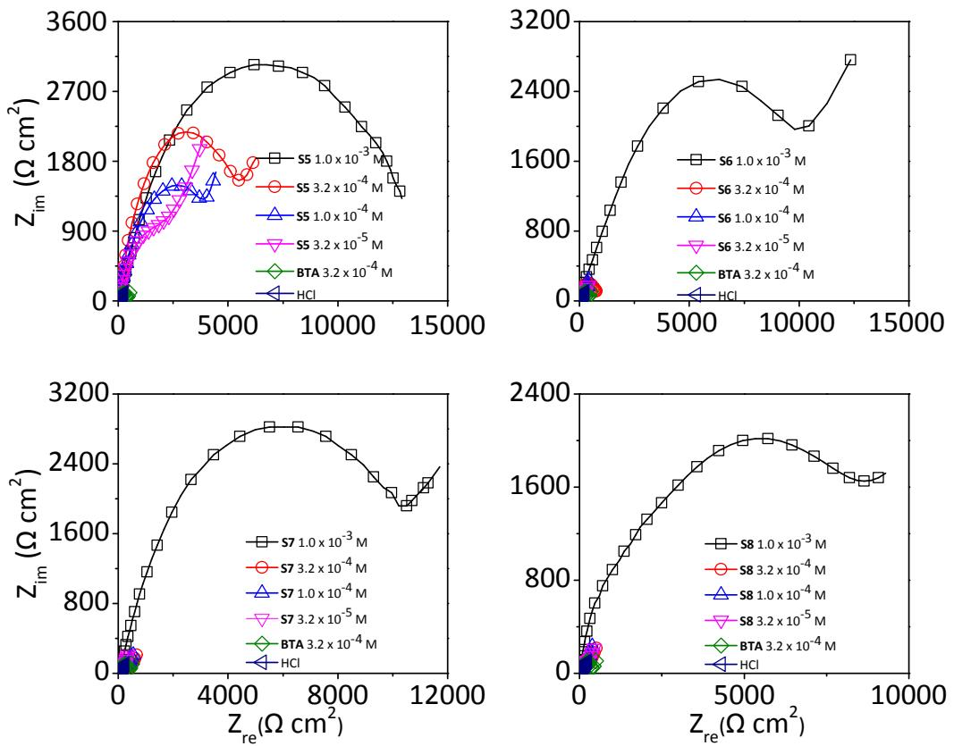
**Figure S4.** Nyquist plots for copper in 1 M HCl in the absence or presence of **S5**, **S6**, **S7** and **S8** of different concentrations with **BTA** as control.
