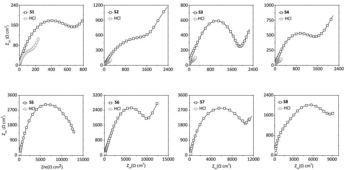
**Figure S2.** Nyquist plots for copper in 1 M HCl in the absence or presence of corrosion inhibitors **S1-S8** ( $10^{-4}$  M).
