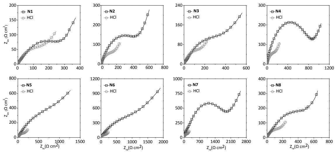
**Figure S3.** Nyquist plots for copper in 1 M HCl in the absence or presence of corrosion inhibitors N1-N8 ( $10^{-4}$  M).
