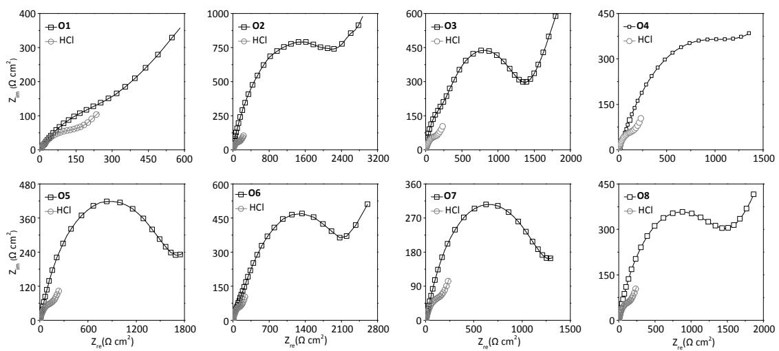
**Figure S1.** Nyquist plots for copper in 1 M HCl in the absence or presence of corrosion inhibitors **O1-O8** ( $10^{-4}$  M).
