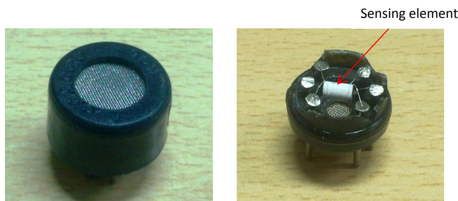
Fig.S1: Packaged CO sensor
