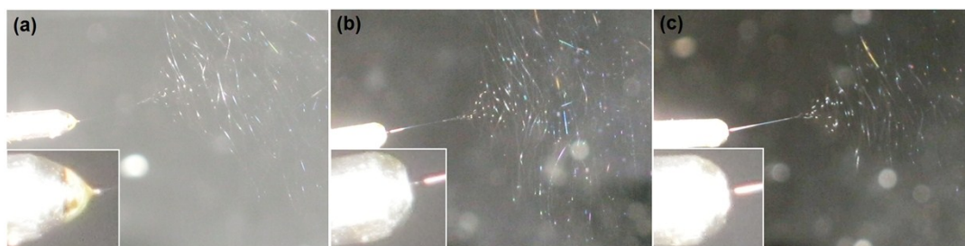
Fig. S2 Digital images of the electrospinning processes for preparing fibers N3 (a), N5 (b) and N6 (c); the insets are the corresponding Taylor cones under an applied voltage of 18 kV.
