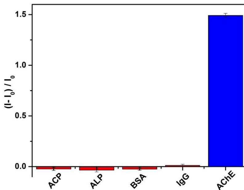
**Figure S11.** Selectivity of the assay toward AChE with comparison to ACP, ALP, BSA, and IgG in buffer solution.  $I_0$  and  $I$  represent the fluorescence intensity before and after the addition of analytes. Activity used for each enzyme is 600.0 U/L.
