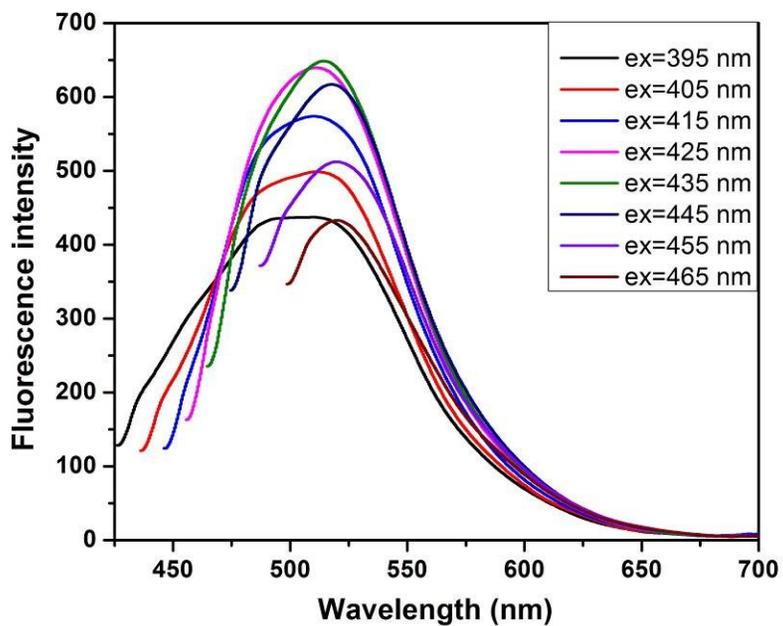
**Figure S4.** Fluorescence spectra of PSA-CQDs nanoprobe with the change of excitation wavelengths in the range of 395 – 465 nm.
