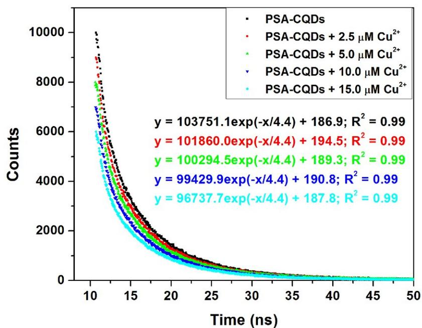
**Figure S5.** Time-resolved decay curves of PSA-CQDs nanoprobe in the presence of different amount of  $\text{Cu}^{2+}$ . The lifetimes are calculated to be 4.4 ns.
