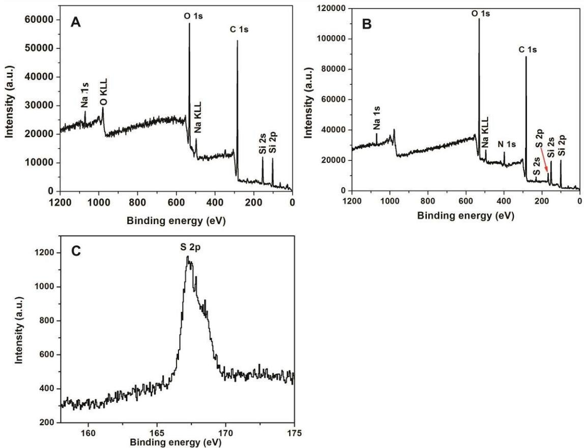
**Figure S2.** Comparison of XPS wide spectra between mere CQDs (A) and PSA-CQDs nanoprobe (B), and high-resolution S2p XPS spectrum for PSA-CQDs nanoprobe (C).
