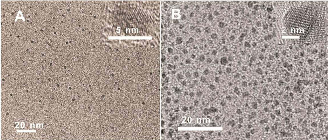
**Figure S1.** (A) TEM image of CQDs. (B) TEM image of PSA-CQDs nanoprobe. Insets: high-resolution TEM images.
