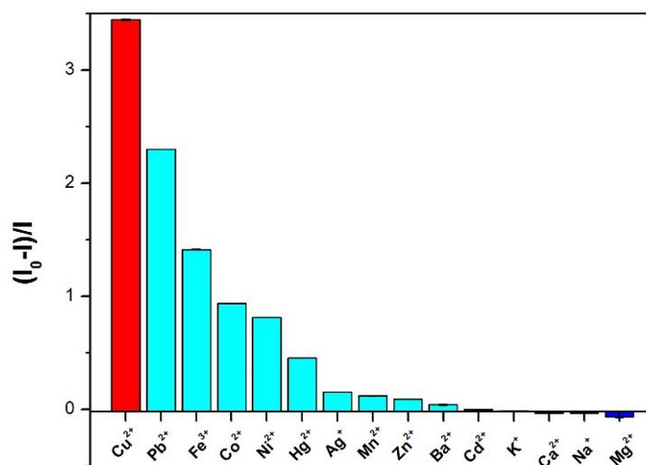
**Figure S6.** The influence of metal cations on the fluorescence of PSA-CQDs nanoprobe. The concentration for each metal ion is 40.0  $\mu\text{M}$ .
