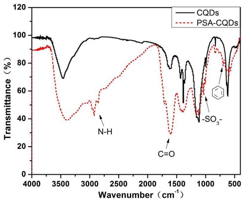
**Figure S3.** IR spectra of PSA-CQDs nanoprobe and CQDs.
