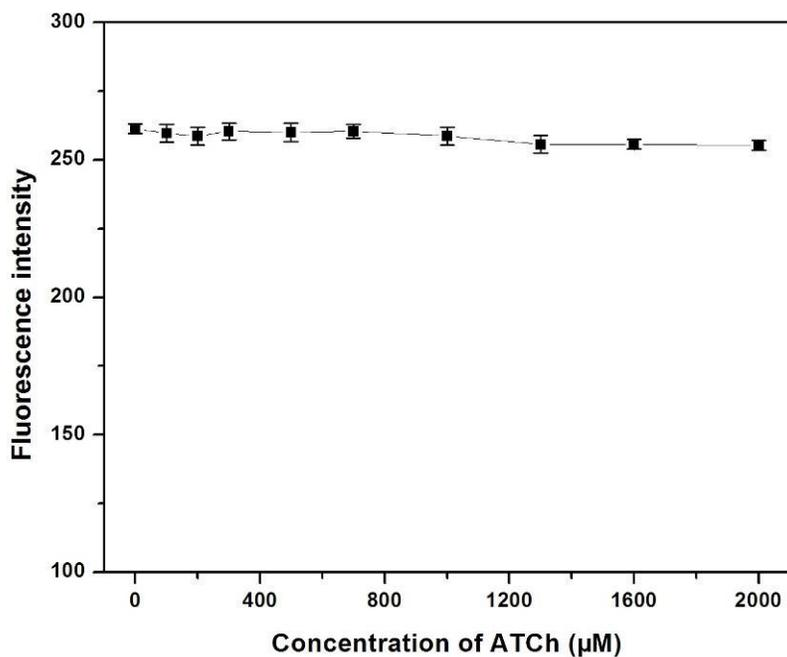
**Figure S8.** The influence of ATCh amount on the fluorescence of PSA-CQDs nanoprobe.
