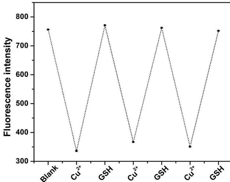
**Figure S10.** The reversibility of PSA-CQDs nanoprobe in response to  $\text{Cu}^{2+}$  and GSH. The concentration for each species is  $20.0 \mu\text{M}$ .
