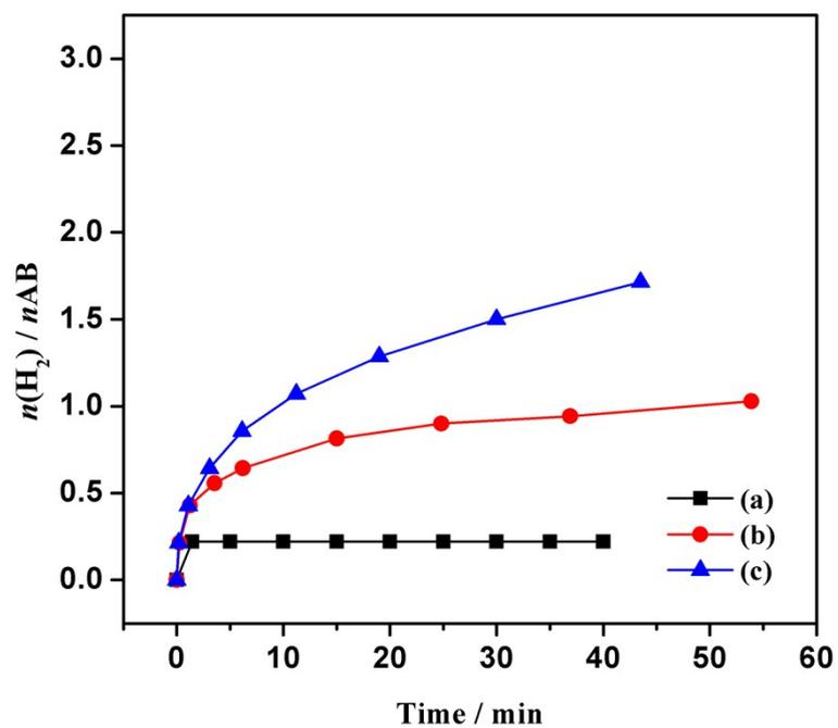
**Fig. S9** Hydrogen generation from the hydrolysis of AB (0.2 M, 5 mL) catalyzed by (a) free Ag, (b) Ag/SiO<sub>2</sub>-12 h, and (c) Ag/SiO<sub>2</sub>-24 h at 298 K (metal/AB = 0.02).
