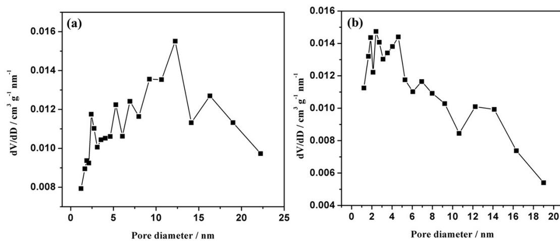
**Fig. S6** The pore size distribution of (a)  $\text{Co@SiO}_2$  and (b)  $\text{Co@SiO}_2/\text{Ag}$  nanospheres.
