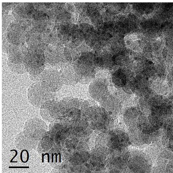
**Fig. S10** TEM image of the recycled Co@SiO<sub>2</sub>/Ag NCs.
