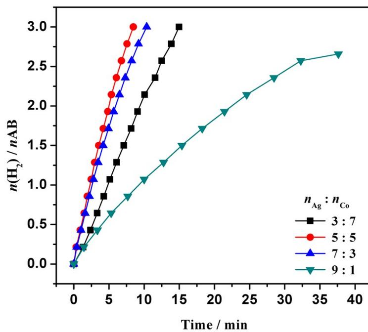
**Fig. S7** Hydrogen generation from the hydrolysis of AB (0.2 M, 5 mL) catalyzed by Co@SiO<sub>2</sub>/Ag NCs with different Ag and Co molar contents at 298 K (metal/AB = 0.02).
