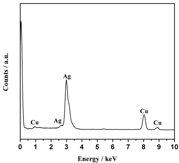
**Fig. S3** The corresponding EDX spectrum for the Ag NPs.
