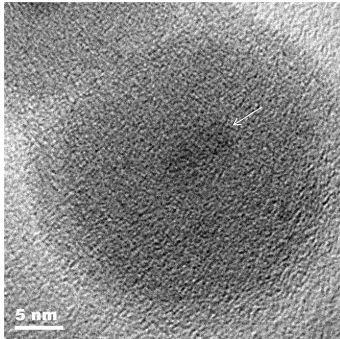
**Fig. S1** TEM image of Co@SiO<sub>2</sub> nanospheres.
