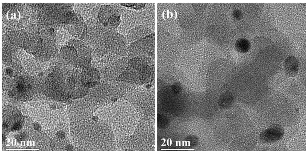
**Fig. S8** TEM images of the (a) Ag/SiO<sub>2</sub>-24 h NCs and (b) Ag/SiO<sub>2</sub>-12 h NCs.
