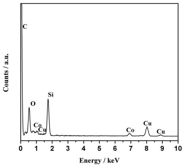
**Fig. S2** The corresponding EDX spectrum for the Co@SiO<sub>2</sub> NPs.
