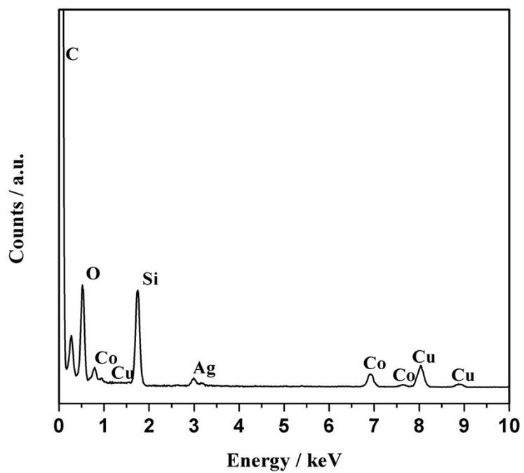
**Fig. S4** The corresponding EDX spectrum for the Co@SiO<sub>2</sub>/Ag NCs.
