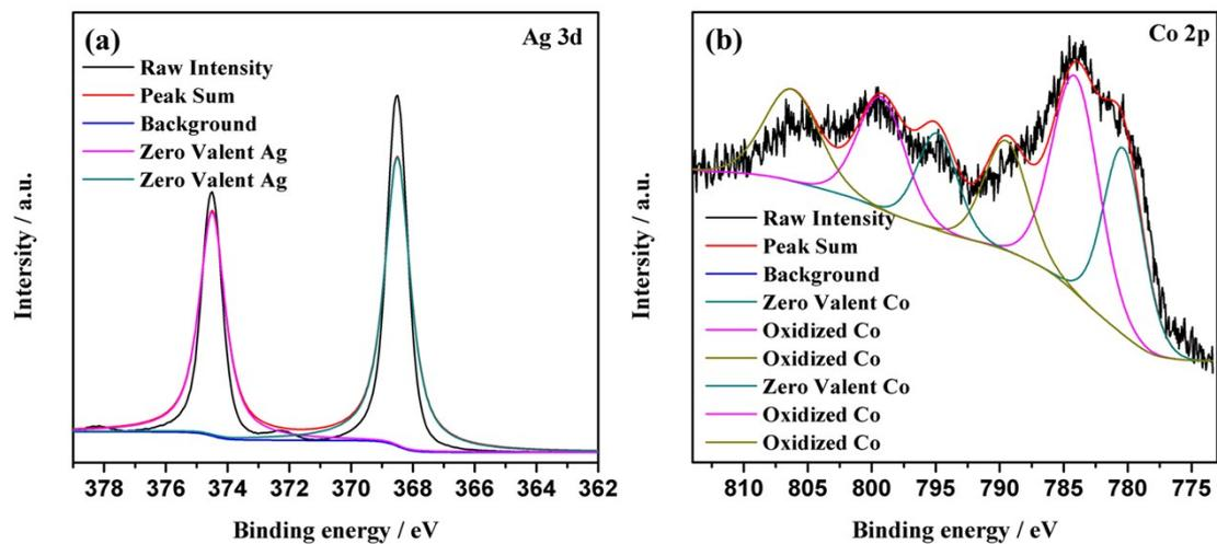
**Fig. S5** XPS spectra of (a) Ag 3d for the free Ag and (b) Co 2p for the Co@SiO<sub>2</sub>.
