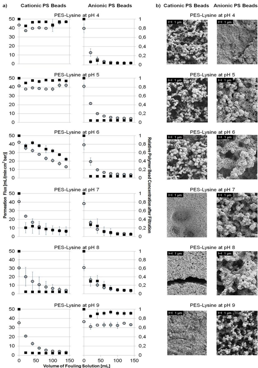
**Figure S9** Fouling of PES-Lysine at different pH values (a) Permeation flux of fouling suspension (left axis, open circles) and normalized concentration of PS beads in filtrate (right axis, filled squares) vs. volume of PS bead suspension; (b) corresponding SEM picture of the membrane after fouling.
