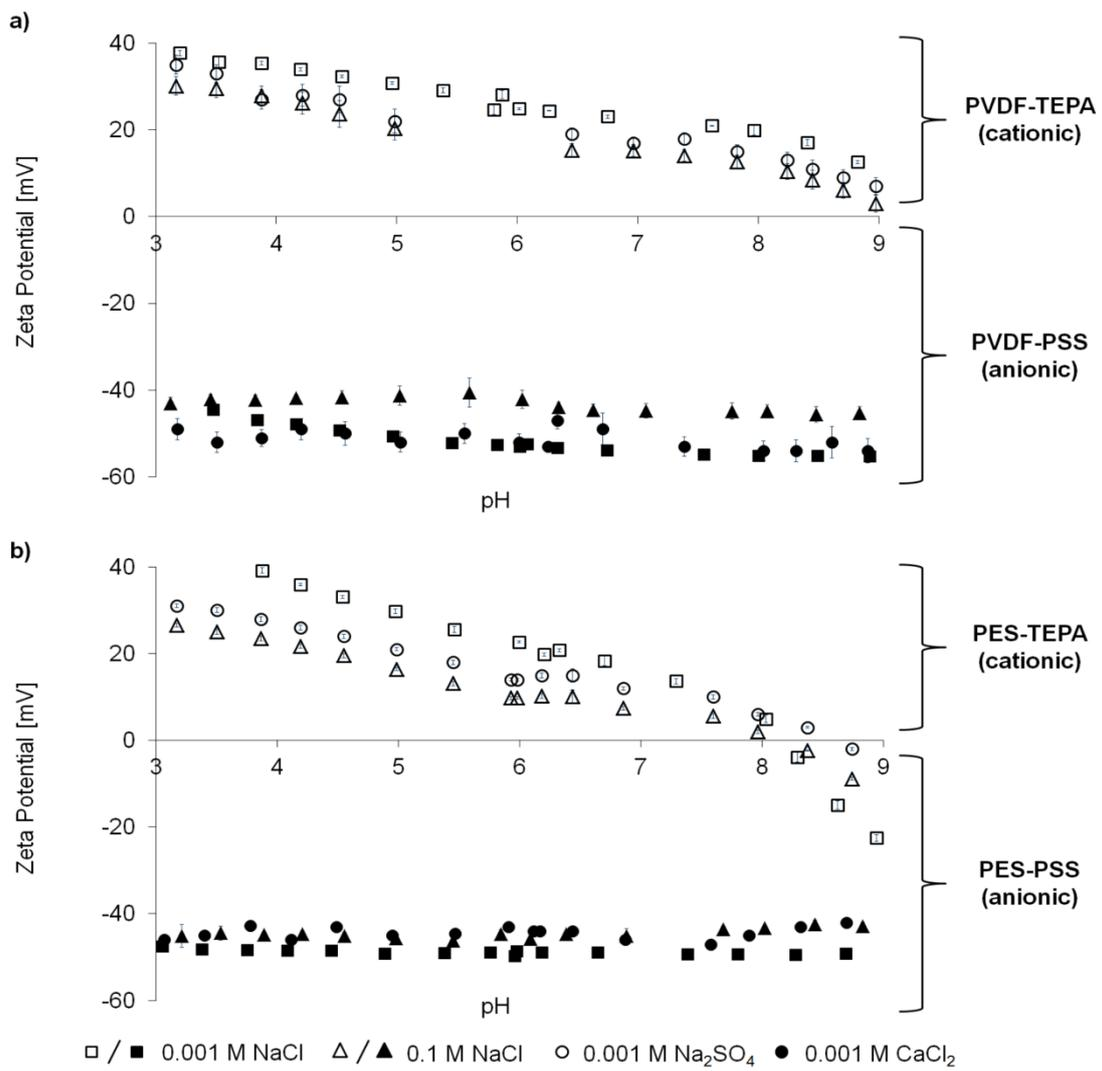
**Figure S4** Zeta potential vs. pH at different salt concentrations of (a) PVDF-TEPA and -PSS membranes; (b) PES-TEPA and -PSS membranes.
