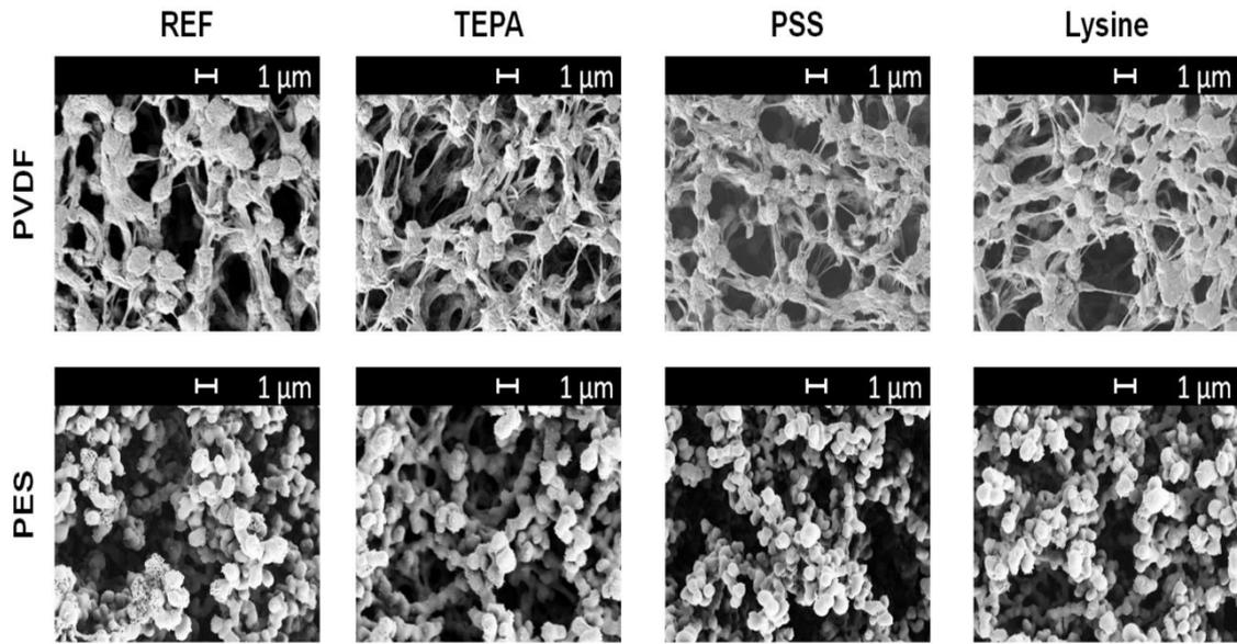
Figure S3 SEM images of modified membranes top side.
