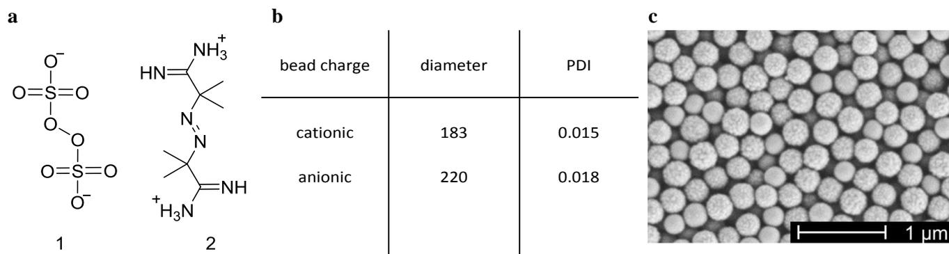
Figure S1 (a) Initiator molecules (1) KPS and (2) AIBA; (b) SEM picture of cationic PS beads, (c) SEM of cationic PS beads.
