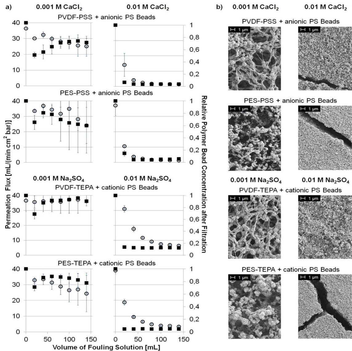
**Figure S6** Repulsive Interactions at 0.001 M and 0.1 M CaCl<sub>2</sub> or Na<sub>2</sub>SO<sub>4</sub>. (a) Permeation flux of fouling suspension (left axis, open circles) and normalized concentration of PS beads in filtrate (right axis, filled squares) vs. volume of PS bead suspension; (b) corresponding SEM picture of the membrane after fouling.
