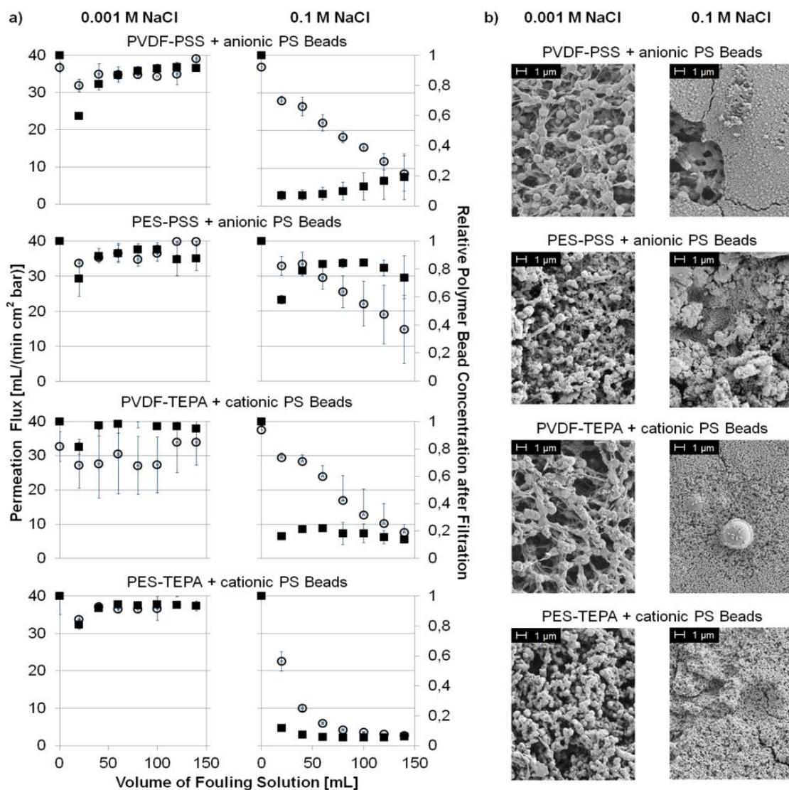
**Figure S5** Repulsive Interactions at 0.001 M and 0.1 M NaCl (a) Permeation flux of fouling suspension (left axis, open circles) and normalized concentration of PS beads in filtrate (right axis, filled squares) vs. volume of PS bead suspension; (b) corresponding SEM picture of the membrane after fouling.
