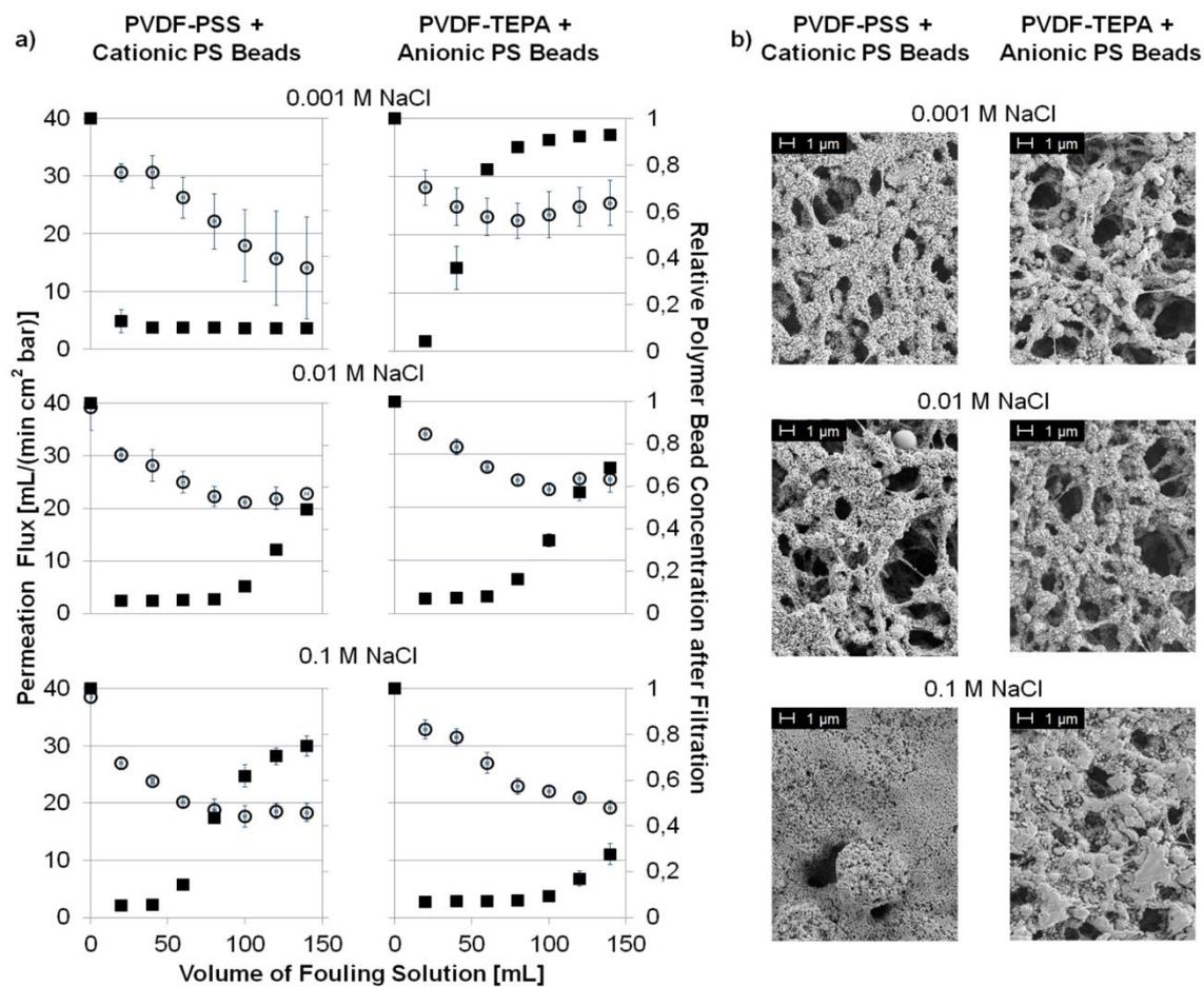
**Figure S8** Attractive Interactions at 0.001 M, 0.01 M, and 0.1 M NaCl (a) Permeation flux of fouling suspension (left axis, open circles) and normalized concentration of PS beads in filtrate (right axis, filled squares) vs. volume of PS bead suspension; (b) corresponding SEM picture of the membrane after fouling.
