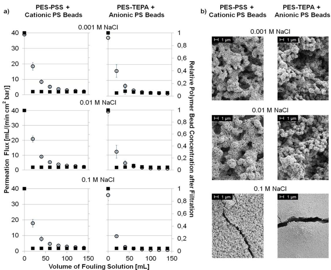
**Figure S7** Attractive Interactions at 0.001 M, 0.01 M, and 0.1 M NaCl (a) Permeation flux of fouling suspension (left axis, open circles) and normalized concentration of PS beads in filtrate (right axis, filled squares) vs. volume of PS bead suspension; (b) corresponding SEM picture of the membrane after fouling.
