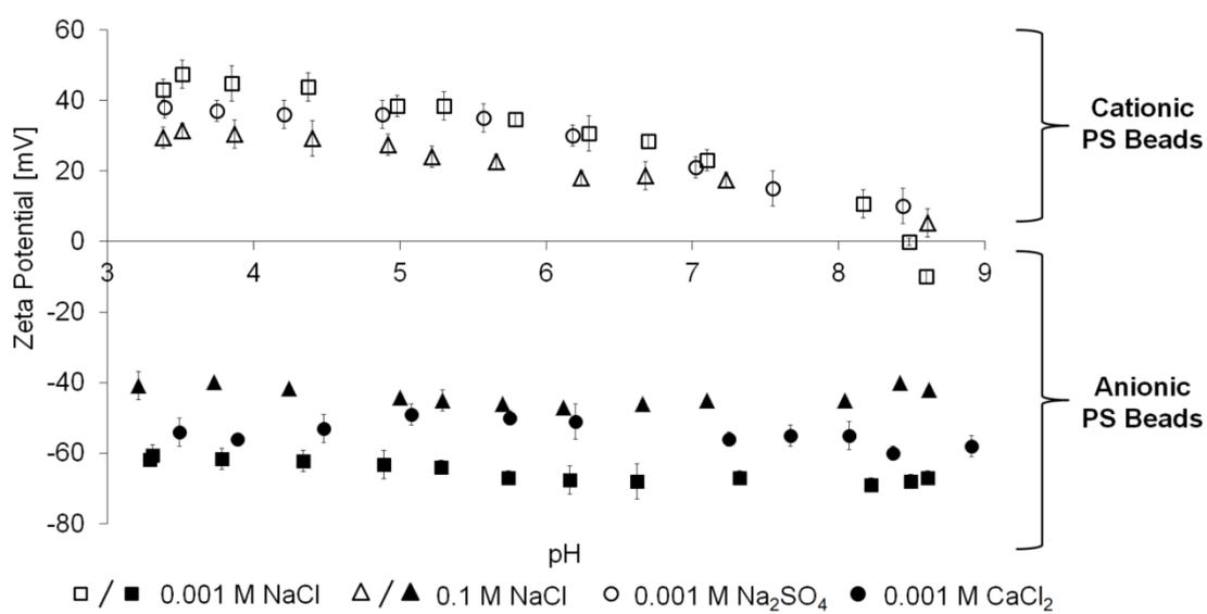
Figure S2 Zeta potential of charged PS beads vs. pH at different salt concentrations.
