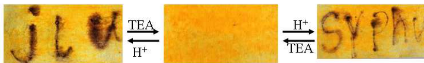
Fig. S8 Photographs of filter papers coated with the ground film of PVBT under different conditions.
