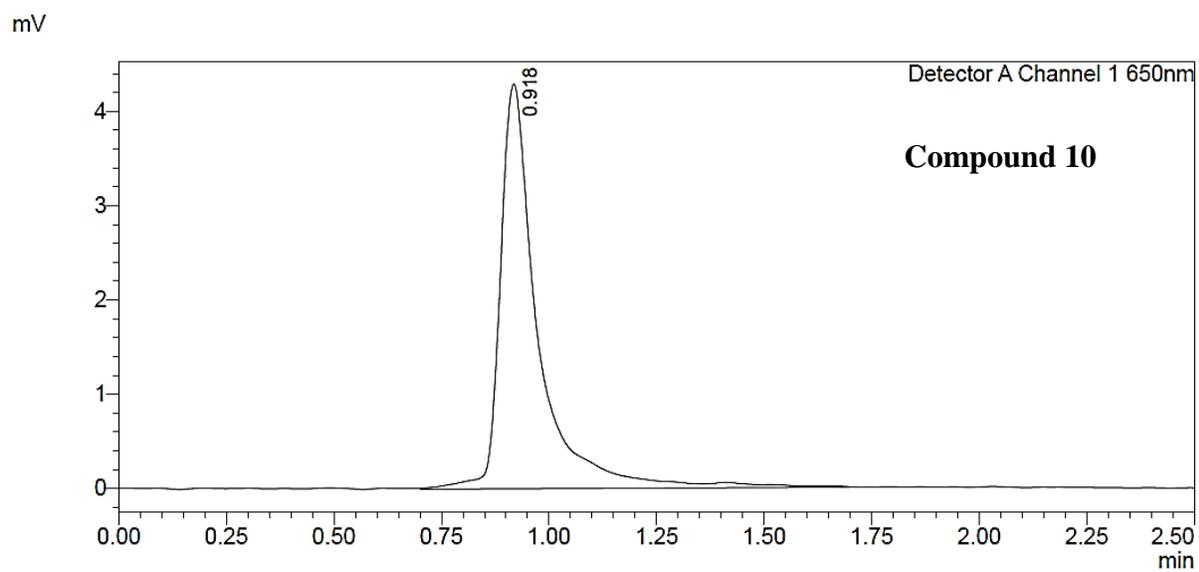
Column: reverse phase HPLC with YMC triart phenyl column and size: 150 × 4.6 mm I.D.,
