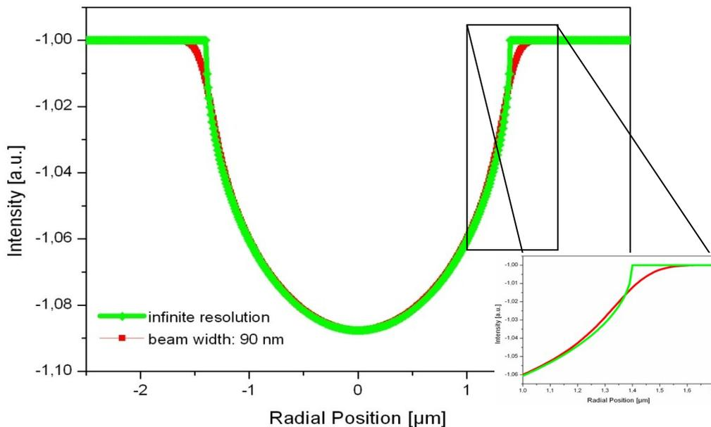
*Fig. S1: Radial transmission profile according to eqn. (2a) – (2c) taking into account infinite STXM resolution and finite beam size. Variations become most obvious at the outermost rim ( $R_1$ ).*
