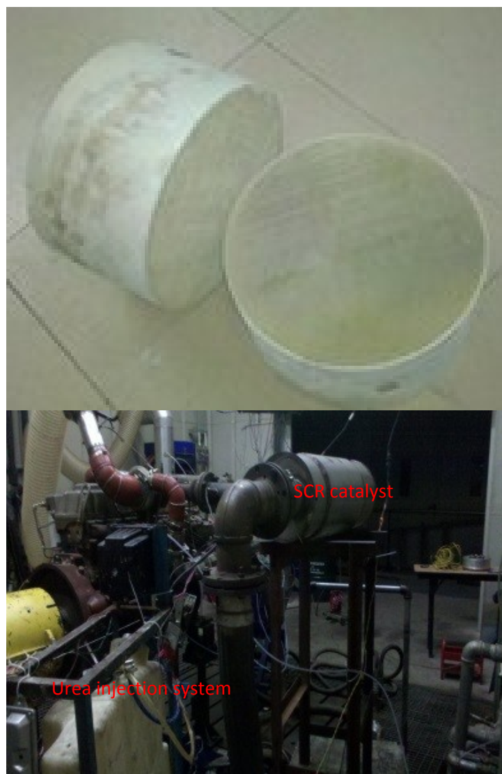
Fig. S2. The engine bench and CuZSM-5-M&CuZSM-5-C honeycomb monoliths catalysts.
