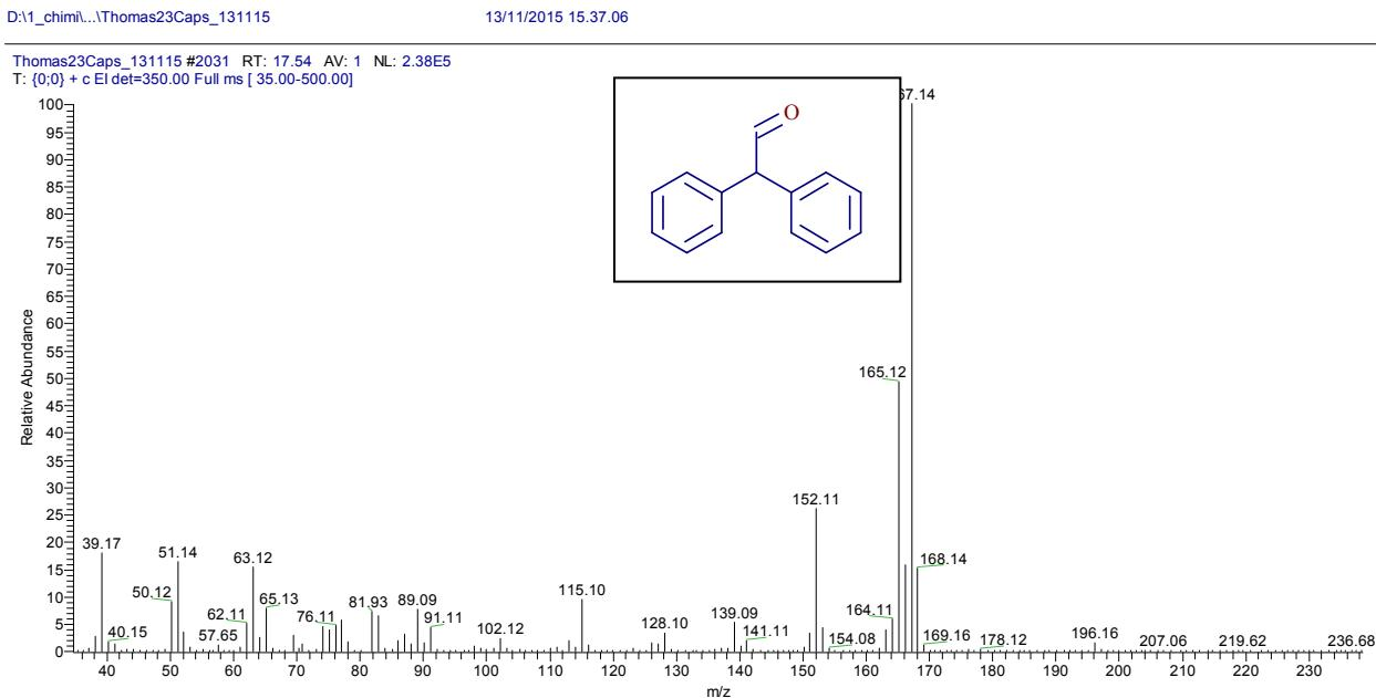
**Figure 7.** Mass spectrum of diphenylacetaldehyde 3h.
