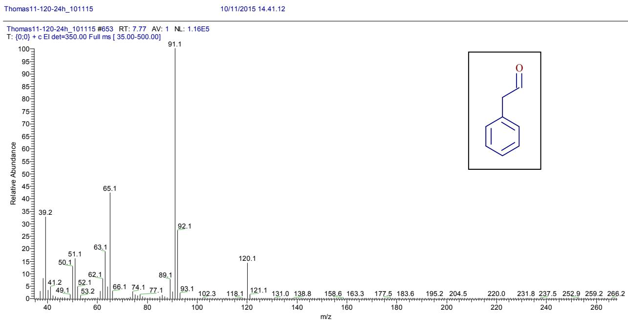
Figure 1. Mass spectrum of phenylacetaldehyde 3a.
