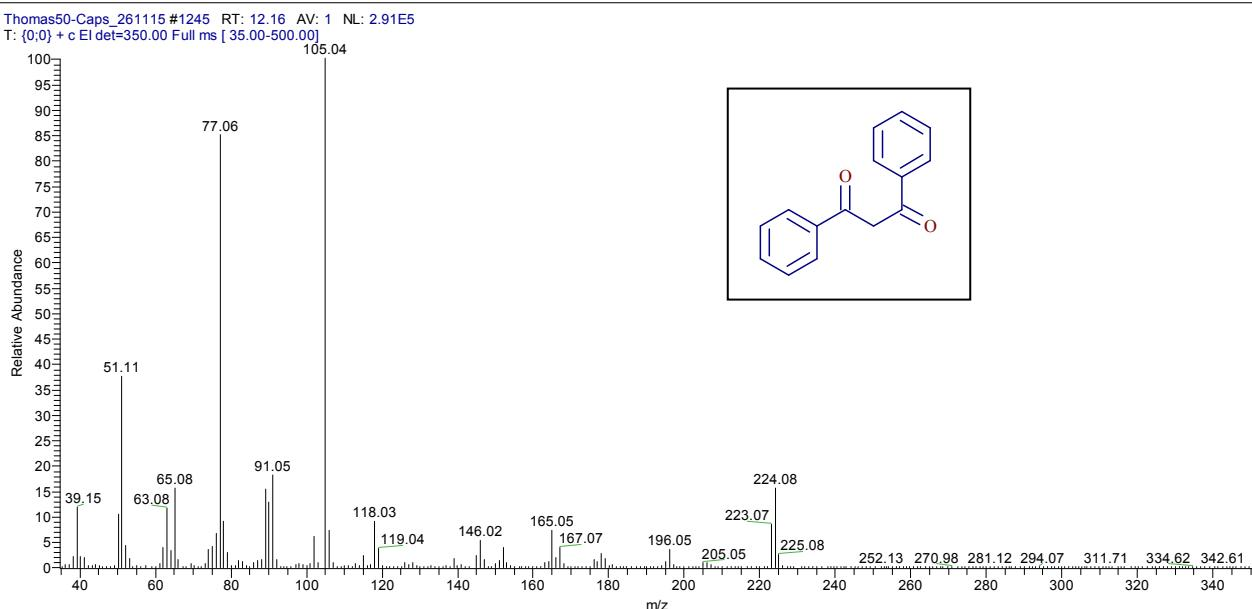
**Figure 11.** Mass spectrum of 1,3-diphenylpropane-1,3-dione **3I'**.
