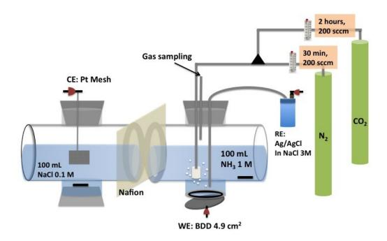
Figure S1. The apparatus for electrochemical reduction of  $CO_2$ .
