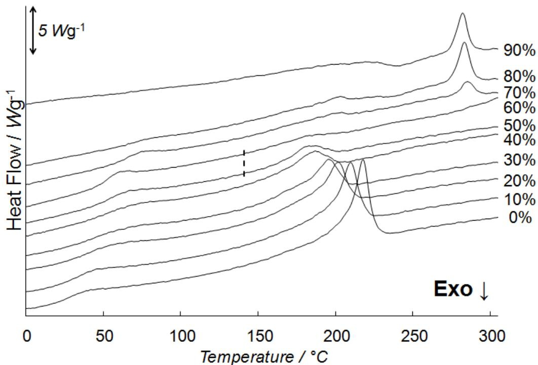
Figure S12: Thermograms of the not actively mixed P3HT-2:PC<sub>61</sub>BM mixtures. The vertical dashed line represents the onset of the melting peaks close to the eutectic. The wt% of PC<sub>61</sub>BM is indicated on the right side of the graph. The curves are shifted vertically for clarity.
