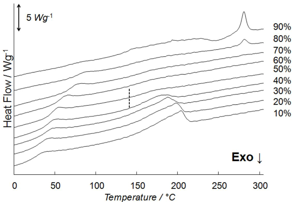
Figure S3: Thermograms of the stirred P3HT-3:PC<sub>61</sub>BM mixtures. The vertical dashed line represents the onset of the melting peaks close to the eutectic. The wt% of PC<sub>61</sub>BM is indicated on the right side of the graph. The curves are shifted vertically for clarity.
