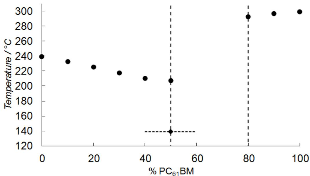
Figure S2: State diagram of stirred P3HT-2:PC<sub>61</sub>BM mixtures. The vertical dashed lines represent the composition range of the eutectic. The horizontal dashed line in the state diagram represents the onset of melting around the eutectic composition.
