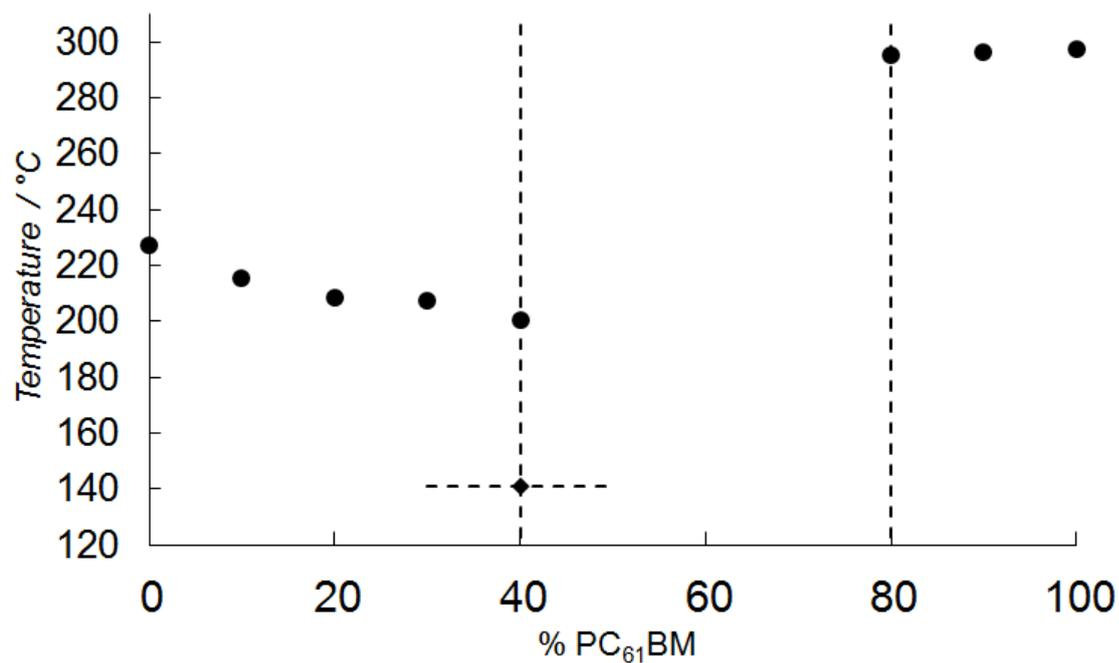
Figure S10: State diagram of sonicated P3HT-3:PC<sub>61</sub>BM mixtures. The vertical dashed lines represent the composition range of the eutectic. The horizontal dashed line in the state diagram represents the onset of melting around the eutectic composition.
