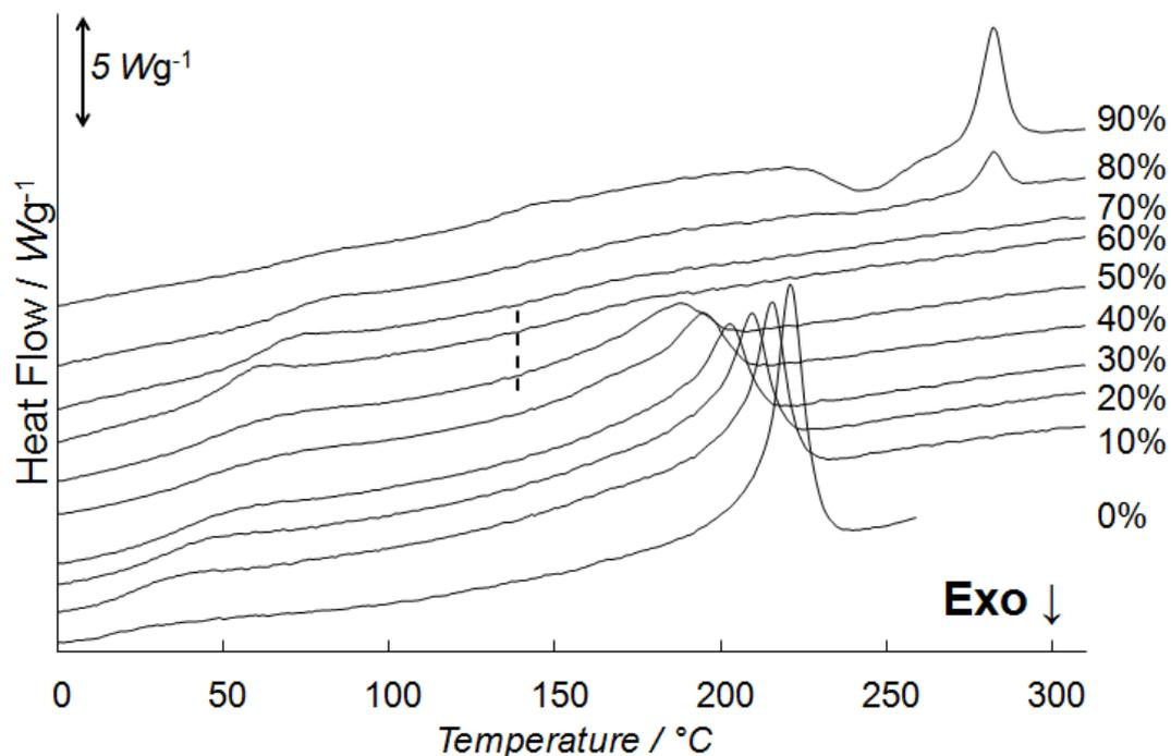
Figure S1: Thermograms of the stirred P3HT-2:PC<sub>61</sub>BM mixtures. The vertical dashed line represents the onset of the melting peaks close to the eutectic. The wt% of PC<sub>61</sub>BM is indicated on the right side of the graph. The curves are shifted vertically for clarity.
