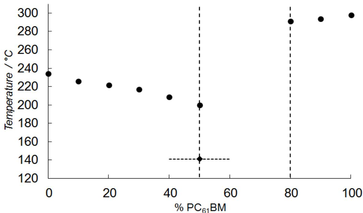
Figure S6: State diagram of sonicated P3HT-1:PC<sub>61</sub>BM mixtures. The vertical dashed lines represent the composition range of the eutectic. The horizontal dashed line in the state diagram represents the onset of melting around the eutectic composition.
