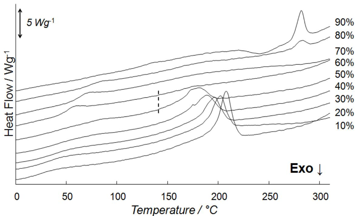
Figure S5: Thermograms of the sonicated P3HT-1:PC<sub>61</sub>BM mixtures. The vertical dashed line represents the onset of the melting peaks close to the eutectic. The wt% of PC<sub>61</sub>BM is indicated on the right side of the graph. The curves are shifted vertically for clarity.
