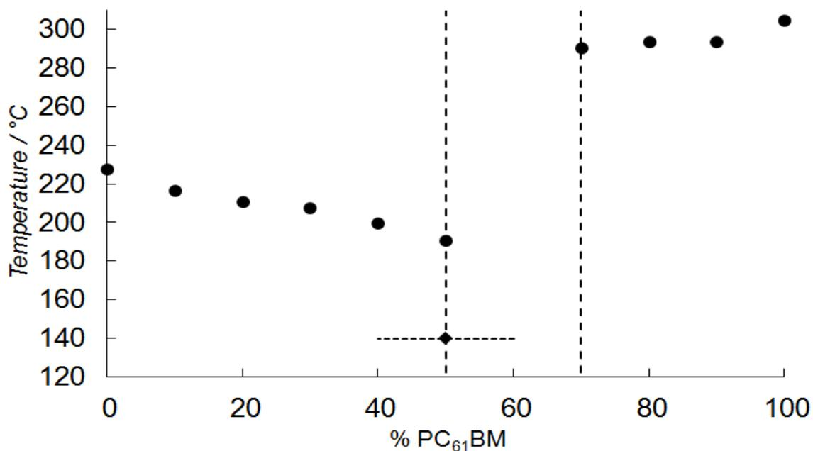
Figure S15: State diagram of not actively mixed P3HT-3:PC<sub>61</sub>BM mixtures. The vertical dashed lines represent the composition range of the eutectic. The horizontal dashed line in the state diagram represents the onset of melting around the eutectic composition.
