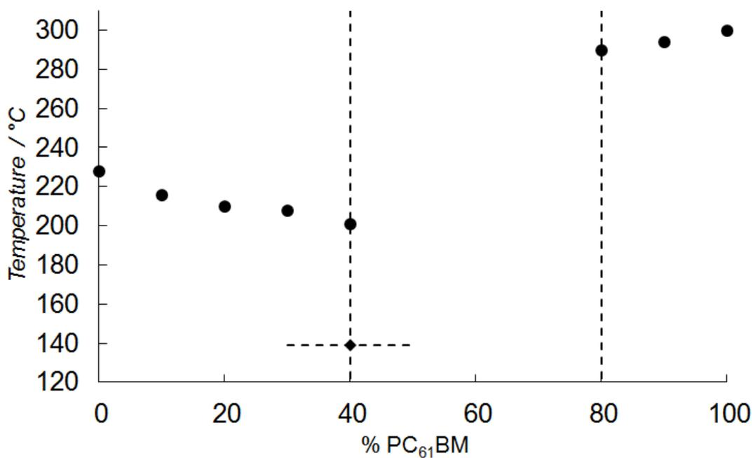
Figure S4: State diagram of stirred P3HT-3:PC<sub>61</sub>BM mixtures. The vertical dashed lines represent the composition range of the eutectic. The horizontal dashed line in the state diagram represents the onset of melting around the eutectic composition.
