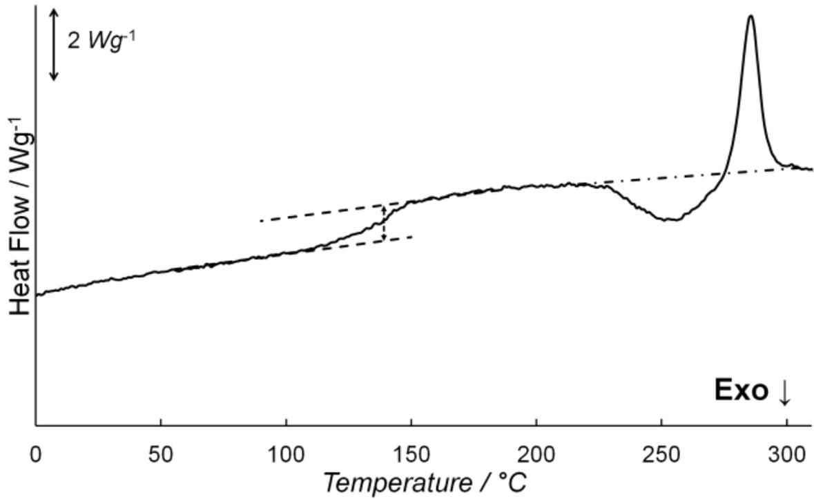
Figure S11: Thermogram of pure virgin PC<sub>61</sub>BM powder obtained at 500 K.min<sup>-1</sup> after cooling at 500 K.min<sup>-1</sup>. The glass transition is situated at 139 °C.
