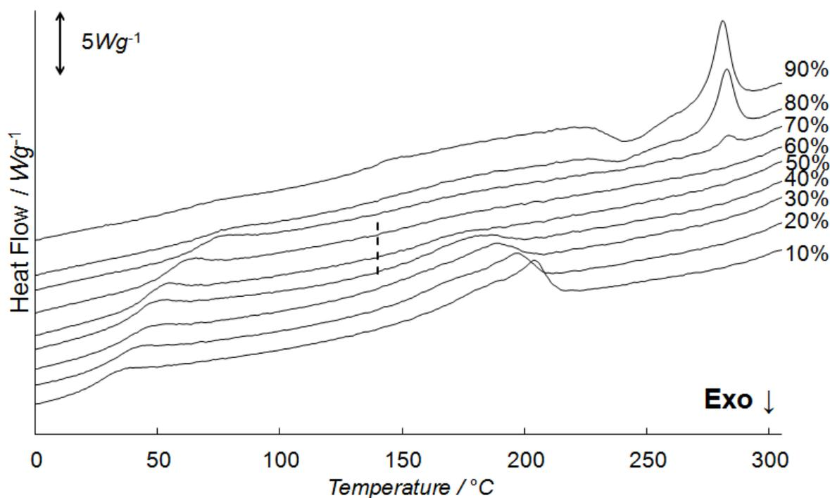
Figure S14: Thermograms of the not actively mixed P3HT-3:PC<sub>61</sub>BM mixtures. The vertical dashed line represents the onset of the melting peaks close to the eutectic. The wt% of PC<sub>61</sub>BM is indicated on the right side of the graph. The curves are shifted vertically for clarity.
