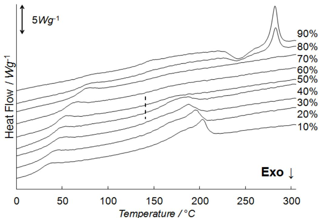
Figure S9: Thermograms of the sonicated P3HT-3:PC<sub>61</sub>BM mixtures. The vertical dashed line represents the onset of the melting peaks close to the eutectic. The wt% of PC<sub>61</sub>BM is indicated on the right side of the graph. The curves are shifted vertically for clarity.
