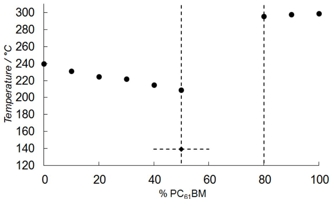
Figure S8: State diagram of sonicated P3HT-2:PC<sub>61</sub>BM mixtures. The vertical dashed lines represent the composition range of the eutectic. The horizontal dashed line in the state diagram represents the onset of melting around the eutectic composition.
