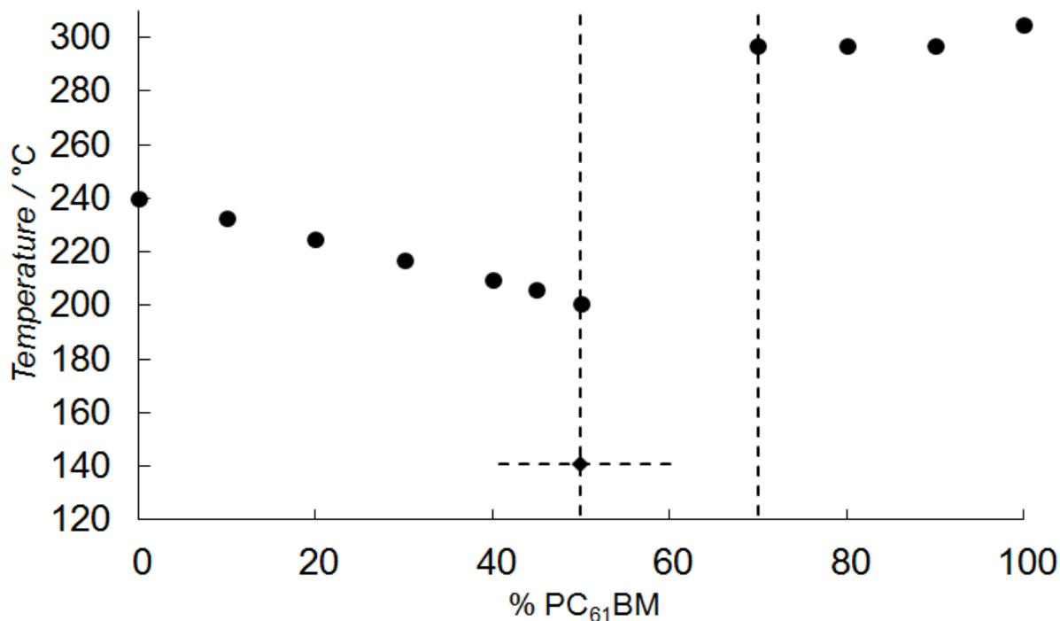
Figure S13: State diagram of not actively mixed P3HT-2:PC<sub>61</sub>BM mixtures. The vertical dashed lines represent the composition range of the eutectic. The horizontal dashed line in the state diagram represents the onset of melting around the eutectic composition.
