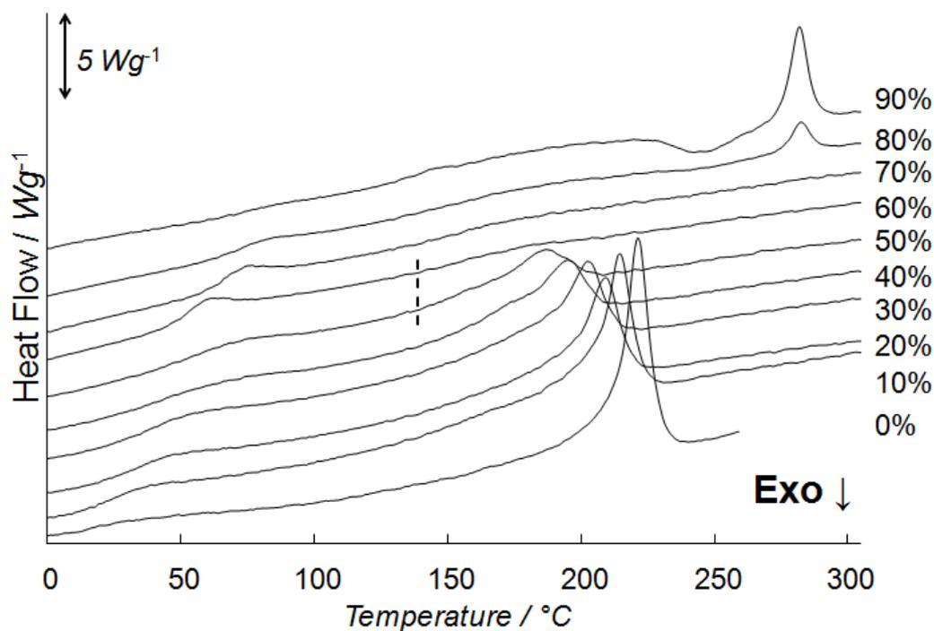
Figure S7: Thermograms of the sonicated P3HT-2:PC<sub>61</sub>BM mixtures. The vertical dashed line represents the onset of the melting peaks close to the eutectic. The wt% of PC<sub>61</sub>BM is indicated on the right side of the graph. The curves are shifted vertically for clarity.
