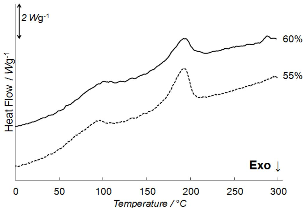
Figure S16: Thermograms of P3HT-2:PC<sub>61</sub>BM mixtures obtained without active mixing at 500 K.min<sup>-1</sup> after cooling at 1 K.min<sup>-1</sup>. The 60 wt% PC<sub>61</sub>BM (full line) represents a mixture that is richer in PC<sub>61</sub>BM compared to the eutectic composition. The 55 wt% PC<sub>61</sub>BM (dashed line) represents a mixture that contains less PC<sub>61</sub>BM than the eutectic composition.
