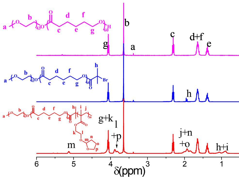
**Fig. S5**  $^1\text{H}$  NMR spectrum of  $\text{PEG}_{43}\text{-}b\text{-PCL}_{60}\text{-}b\text{-PTMA}_{30}$  (L1).
