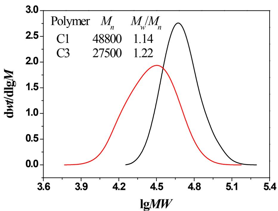
**Fig. S7** GPC traces of C3 after reduction of C1 to cleave the disulfide linkage.
