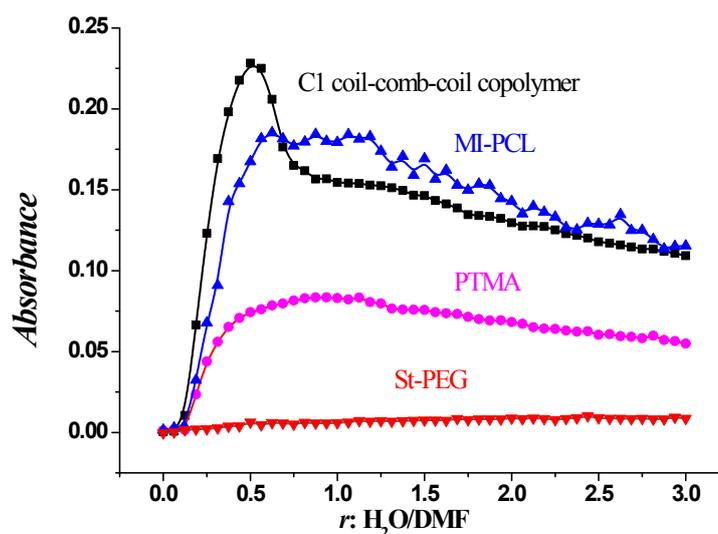
**Fig. S4** The turbidity studies in the mixture solution of H<sub>2</sub>O/DMF ( $r$ , v/v) of C1 coil-comb-coil copolymer and corresponding homopolymers of St-PEG, MI-PCL and PTMA with the same concentration as that of C1 during self-assembly.
