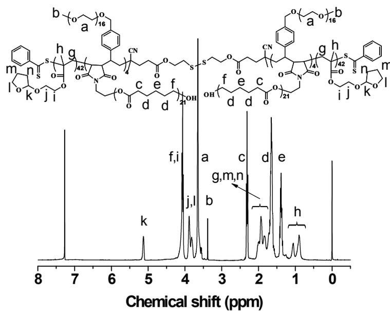
**Fig. S2**  $^1\text{H}$  NMR spectrum of PTMA<sub>42</sub>-*b*-[(St-PEG<sub>16</sub>)-*alt*-(MI-PCL<sub>21</sub>)]<sub>4</sub>-S-S-[(St-PEG<sub>16</sub>)-*alt*-(MI-PCL<sub>21</sub>)]<sub>4</sub>-*b*-PTMA<sub>42</sub> copolymer (C1).
