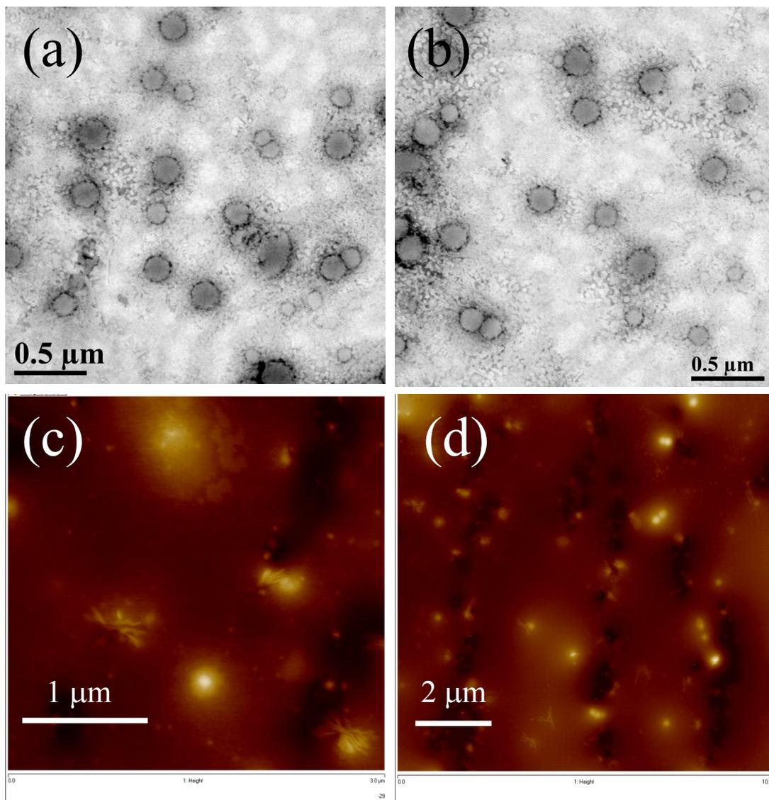
**Fig. S3** Additional TEM (a-b) and AFM (c-d) images of C1 hairy nanoparticles at  $r = 2:1$ .
