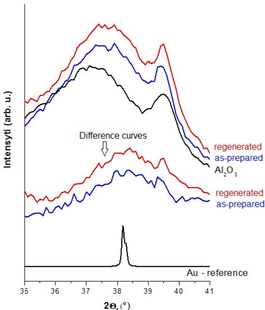
**Figure S1.** Fragments of X-ray diffraction patterns for as-prepared and regenerated Au/Al<sub>2</sub>O<sub>3</sub> catalyst.
