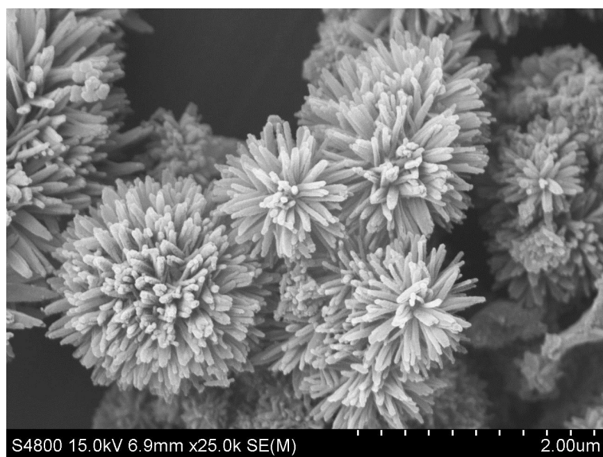
Fig. S2. SEM image of nitrogen-doped hollow carbon nanoflowers (N-HCNFs).
