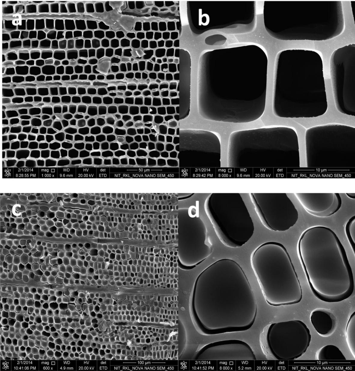
Figure S2: Microstructure of the SiCo ceramics pyrolyzed at 900 °C; (a, b) infiltrated once with the preceramic polymers, (c, d) samples with 5 infiltration cycles.
