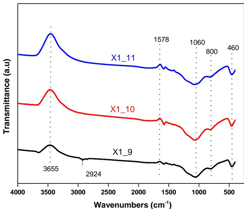
Figure S3: FTIR spectra for X1 pyrolysed at different pyrolysis temperature (900-1100 °C)
