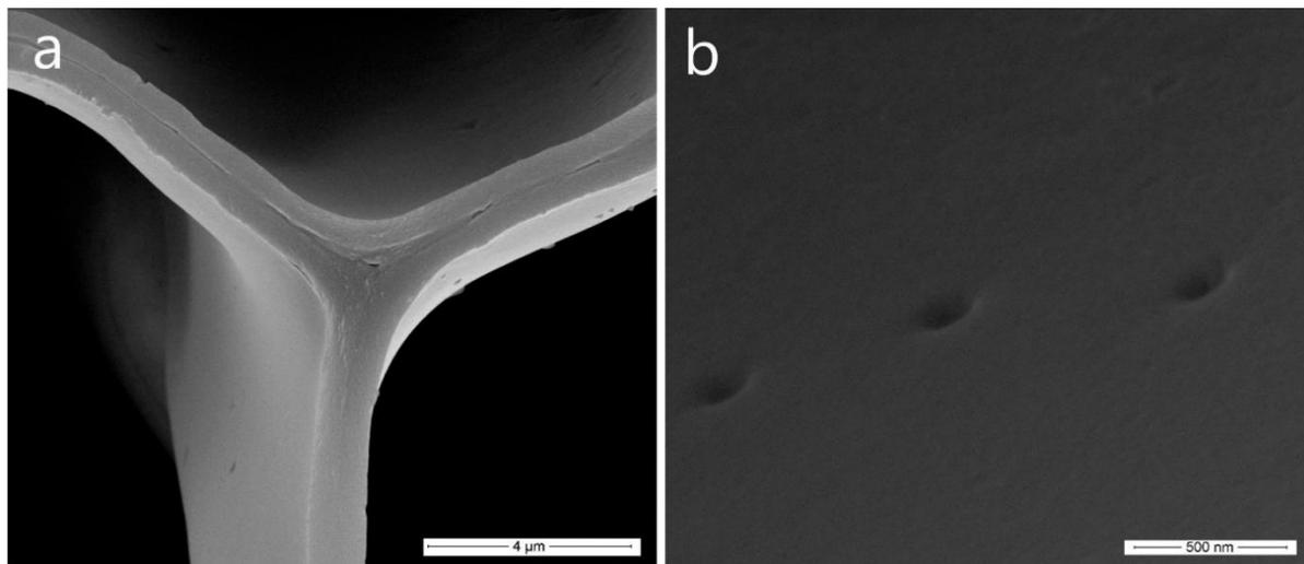
Figure S4: (a) Strut details of X1 sample pyrolyzed at 900 °C, (b) Strut interior
