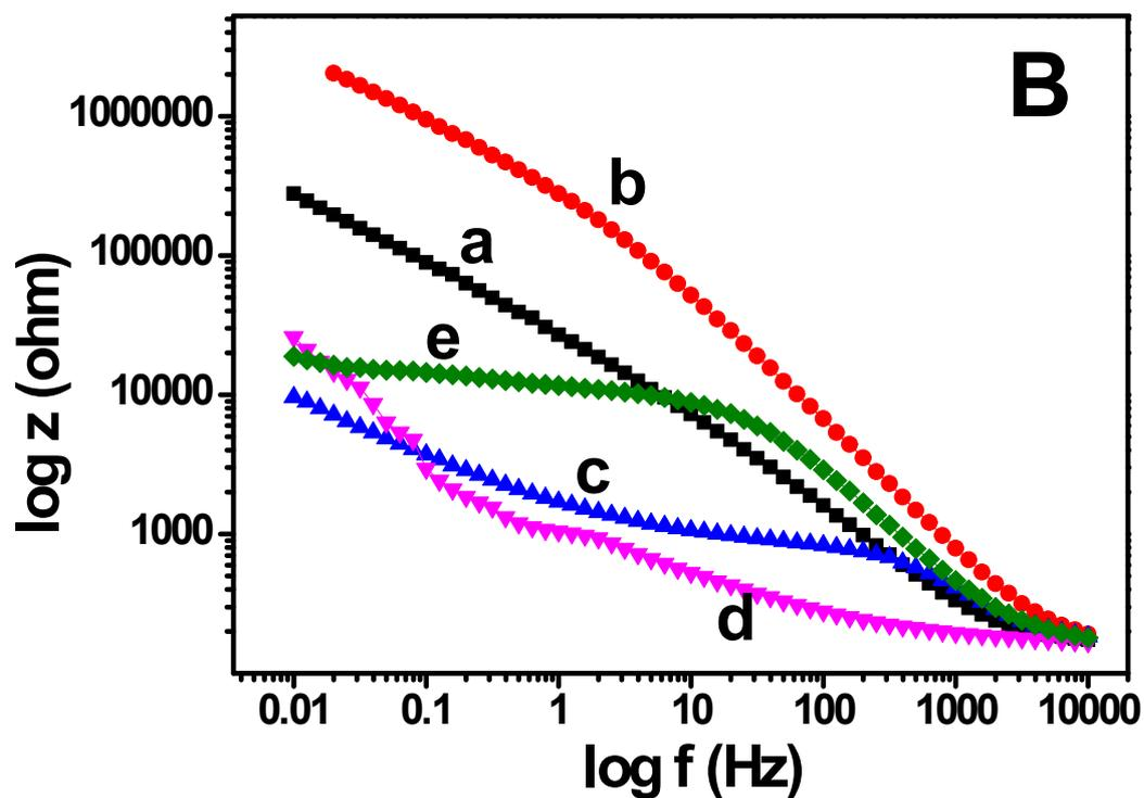
**Fig. S2 (A)** Bode phase plots obtained for bare GC (a) GO (b), rGO-Ag (0.5 M) (c), rGO-Ag (1.0 M) (d) and rGO-Ag (5.0 M) (e) modified GC electrodes for 1 mM  $K_3[Fe(CN)_6]$  in 0.1 M KCl. **(B)** Bode impedance plots ( $\log Z$  vs.  $\log f$ ) obtained for bare GC (a) GO (b), rGO-Ag (0.5 M) (c), rGO-Ag (1.0 M) (d) and rGO-Ag (5.0 M) (e) modified GC electrodes for 1 mM  $K_3[Fe(CN)_6]$  in 0.1 M KCl.
