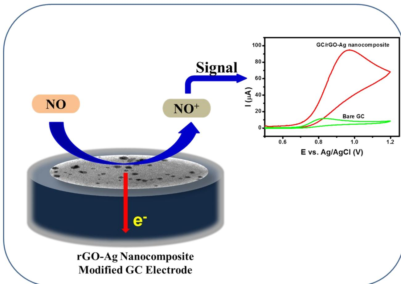
**Scheme S1.** Graphical illustration of NO electrooxidation at the rGO-Ag (5.0 M) nanocomposite modified GC electrode.
