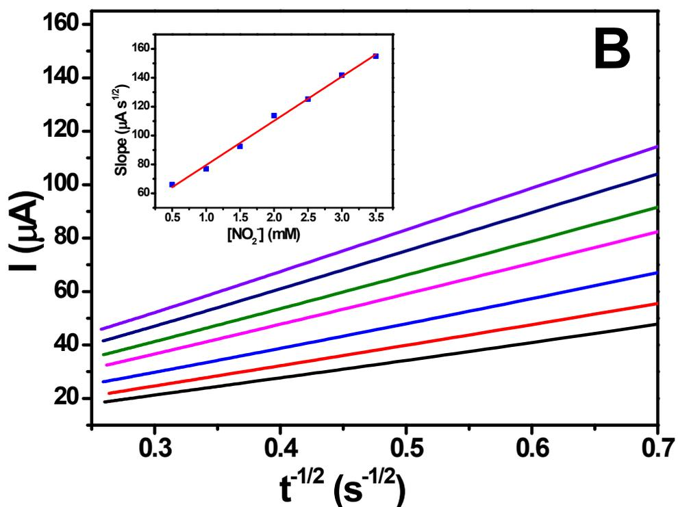
**Fig. S8** Chronoamperograms obtained at rGO-Ag (5.0 M) nanocomposite modified electrode with different concentrations of  $\text{NO}_2^-$  in 0.1 M phosphate buffer (pH 2.5). Applied potential was +0.96 V (A) and plot of current versus  $t^{-1/2}$  (B). Inset: Plot of slopes obtained from straight lines of 'B' versus concentration of  $\text{NO}_2^-$ .
