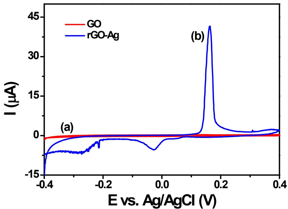
**Fig. S3** Cyclic voltammogram recorded at GO (a) and rGO-Ag (5.0 M) nanocomposite (b) modified electrode in 0.1 M phosphate buffer (pH 2.5) with scan rate of 50 mV s<sup>-1</sup>.
