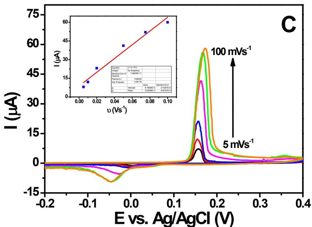
**Fig. S4** Cyclic voltammograms recorded at rGO-Ag (A: 0.5 M, B: 1.0 M and C: 5.0 M) nanocomposite modified electrodes in  $N_2$ -saturated 0.1 M phosphate buffer (pH 2.5) with different scan rates (5-100  $mV s^{-1}$ ) and inset shows the plot of anodic peak current versus scan rate.
