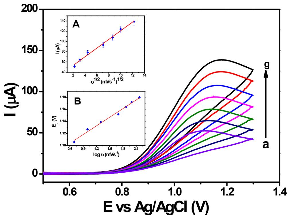
**Fig. S7** Cyclic voltammograms recorded at rGO-Ag (5.0 M ascorbic acid) nanocomposite modified electrode for 5 mM of  $\text{NO}_2^-$  in 0.1 M phosphate buffer (pH 2.5) with various scan rates (a: 5, b: 10, c: 20, d: 50, e: 75, f: 100 and g: 150  $\text{mV s}^{-1}$ ). Inset: Plot of peak current versus square root of scan rate (A) and plot of peak potential versus log (scan rate) (B).
