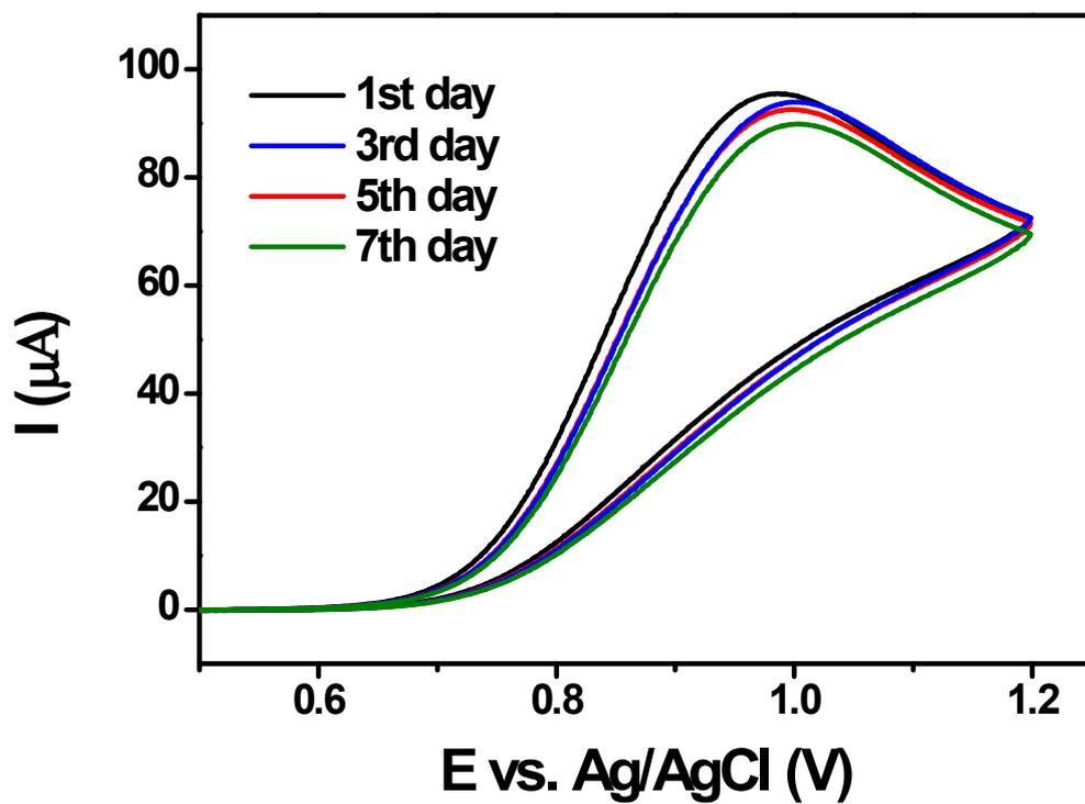
**Fig. S5** Cyclic voltammograms recorded for 1 mM NO<sub>2</sub><sup>-</sup> at the GC/rGO-Ag (5.0 M) nanocomposite modified electrode during different days in 0.1 M PBS (pH 2.5) with a scan rate of 50 mV s<sup>-1</sup>.
