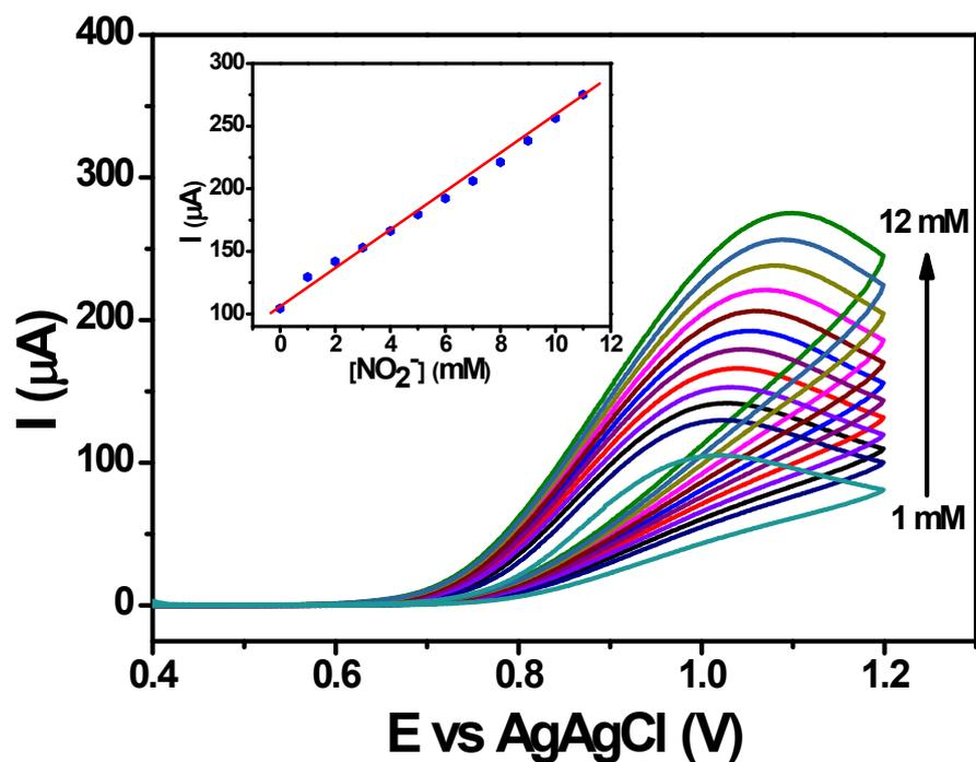
**Fig. S6** Cyclic voltammograms obtained at the rGO-Ag (5.0 M) nanocomposite modified electrode for the successive addition of each 1 mM of  $\text{NO}_2^-$  (1-12 mM) in 0.1 M phosphate buffer (pH 2.5) with a scan rate of  $50 \text{ mV s}^{-1}$ . Inset: Plot of peak current versus concentration of  $\text{NO}_2^-$ .
