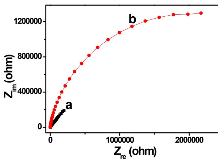
**Fig. S1** Nyquist plots obtained for bare GCE (a) and GO (b) for 1 mM  $K_3[Fe(CN)_6]$  in 0.1 M KCl.
