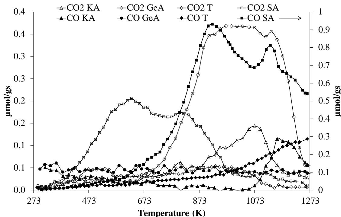
Figure S1.  $\text{CO}_2$  and  $\text{CO}$  evolution in TPD experiments carried out with the carbon materials used as support
