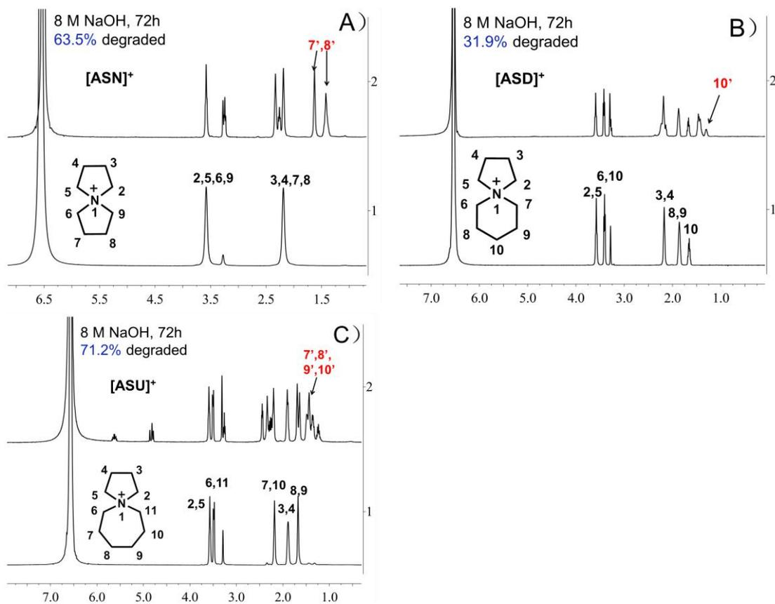
**Figure S2.**  $^1\text{H}$ NMR spectra of (A)  $[\text{ASN}]^+$ , (B)  $[\text{ASD}]^+$ , (C)  $[\text{ASU}]^+$  in 8 M NaOH  $\text{CD}_3\text{OD}/\text{D}_2\text{O}$  solution ( $V_{\text{CD}_3\text{OD}}:V_{\text{D}_2\text{O}}=3:1$ ) at 80 °C for 72 h.
