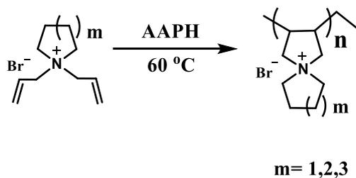
**Scheme S1.** Synthesis of spirocyclic QA cation based polymers.
