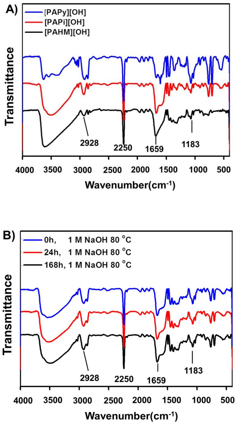
**Figure S3.** FT-IR of A) [PAPy][OH], [PAPi][OH], and [PAHM][OH] membranes; B) [PAPi][OH] membrane in 1M NaOH at 80 °C for various time.
