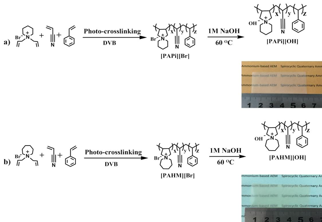
**Scheme S2.** Synthetic routes of Spiroheterocyclic Quaternary Ammonium-Based Anion Exchange Membranes and the photographs of [PAPi][OH], and [PAHM][OH]. The membranes are transparent, flexible, and could be easily cut into desired sizes.
