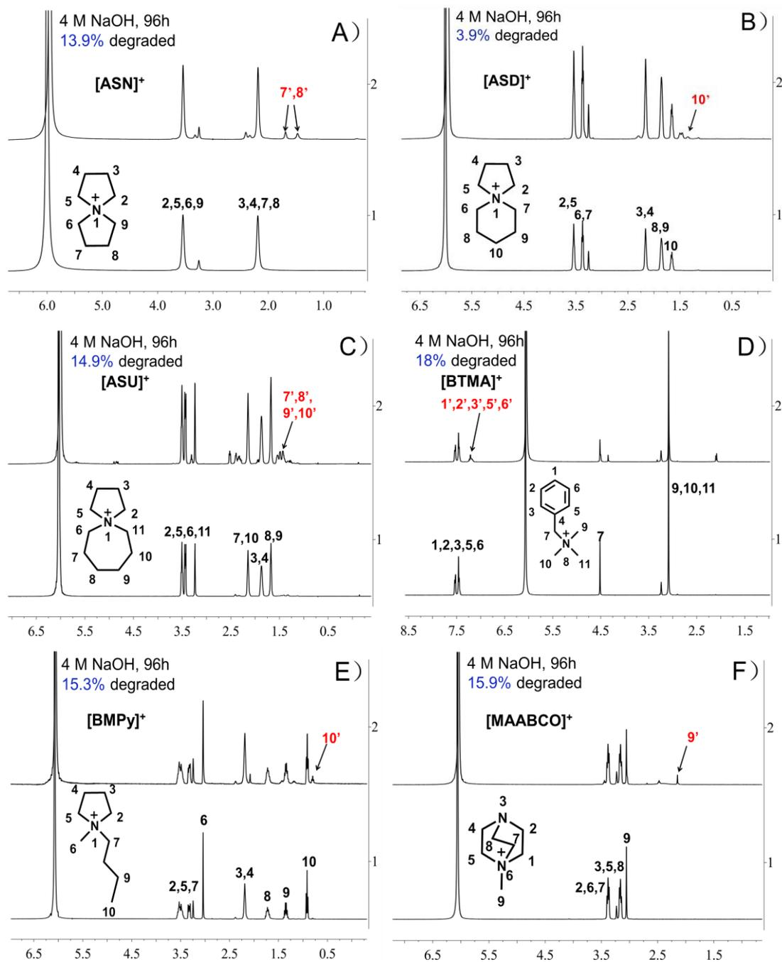
**Figure S1.**  $^1\text{H}$ NMR spectra of (A) [ASN] $^+$ , (B) [ASD] $^+$ , (C) [ASU] $^+$ , (D) [BTMA] $^+$ , (E) [BMPy] $^+$ , (F) [MAABCO] $^+$  in 4 M NaOH  $\text{CD}_3\text{OD}/\text{D}_2\text{O}$  solution ( $V_{\text{CD}_3\text{OD}}:V_{\text{D}_2\text{O}}=3:1$ ) at  $80^\circ\text{C}$  for 96 h.
