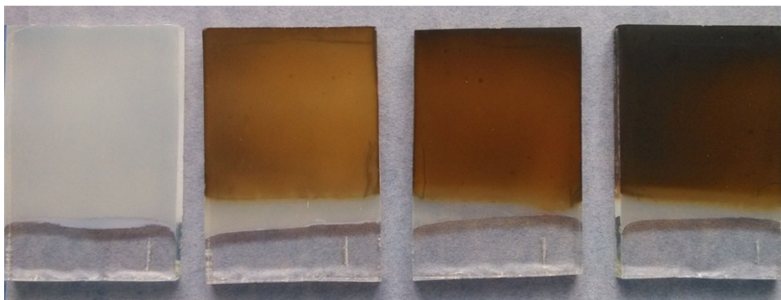
Fig. S2 Digital photos of the ZnO/Cu 2 SnS 3 nanorod arrays films with different deposition time of 0 s, 60 s, 90 s and 120 s.
