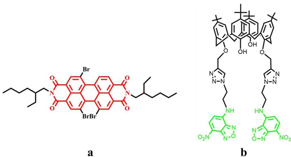
**Figure S1** Molecular structures of the fluorescent probes employed: a) perylene bisimide derivative 1; b) NBD derivative 2.
