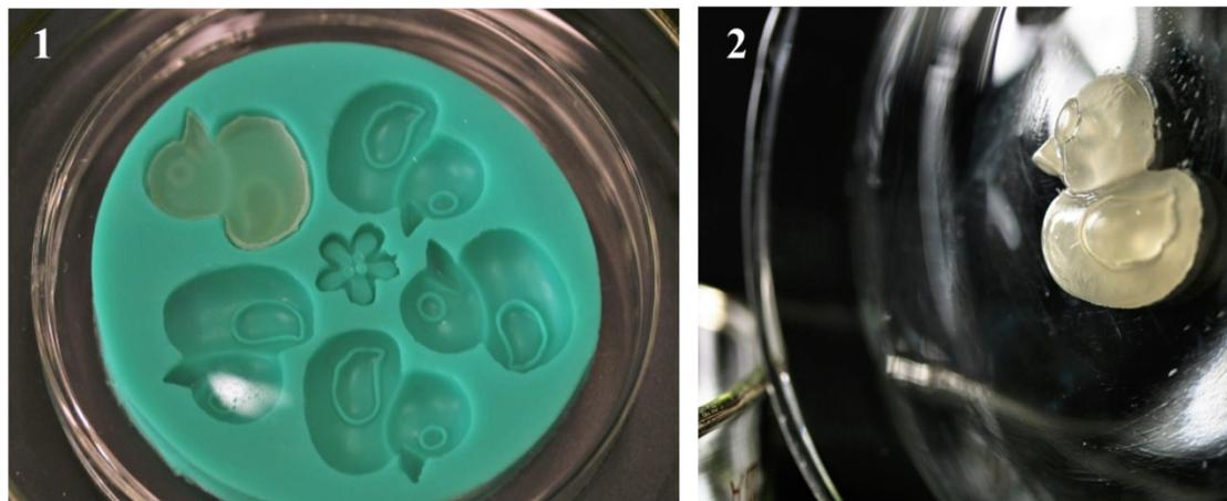
Figure S6 A 'duck' modeled with the CTA/PTMS gel.
