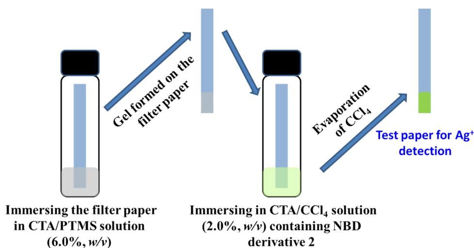
**Figure S5** Schematic representation of the fabrication of a test paper for Ag<sup>+</sup> detection.
