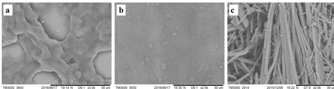
Figure S3 SEM images of the xerogels of CTA from: a) PTMS, b) PTES, and c)  $\text{CCl}_4$ .
