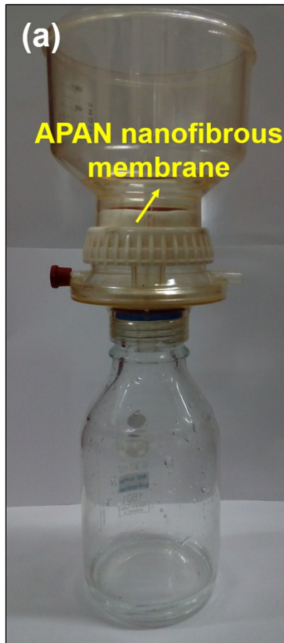
Fig.S3 (a) Experimental setup of filtration unit
