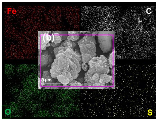
**Figure S3.** (a) EDS spectra and (b) EDS mapping images for a selected region of Basolite F300.
