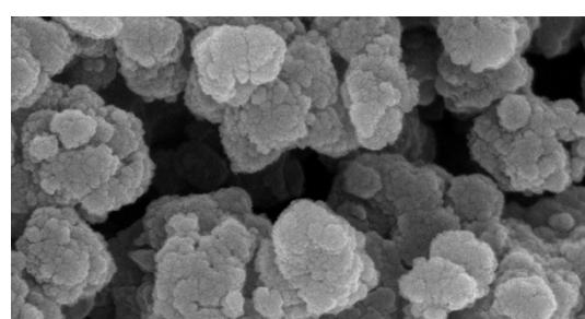
**Figure S6.** High-resolution SEM imagine of the synthetic Fe-BTC material.
