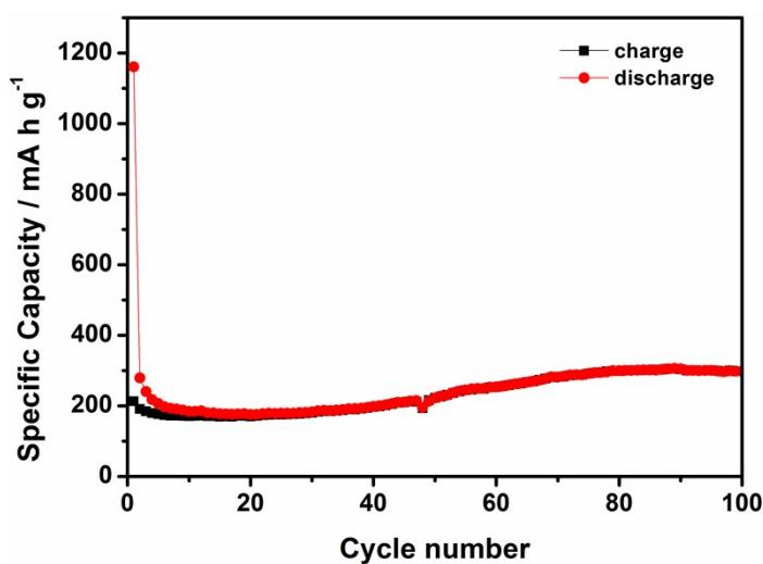
**Figure S8.** Cycling performance of the bulk material Basolite F300 at the current density of  $500 \text{ mA g}^{-1}$ .
