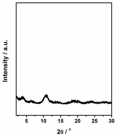
**Figure S2.** PXRD pattern of Fe-BTC product obtained using  $\text{FeCl}_3 \cdot 6\text{H}_2\text{O}$  as the iron source.
