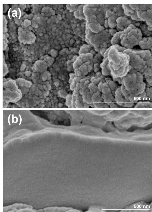
**Figure S5.** High-resolution SEM imagines of Basolite F300: enlargements of the (a) top and (b) left bottom particles of Figure 5a, respectively.
