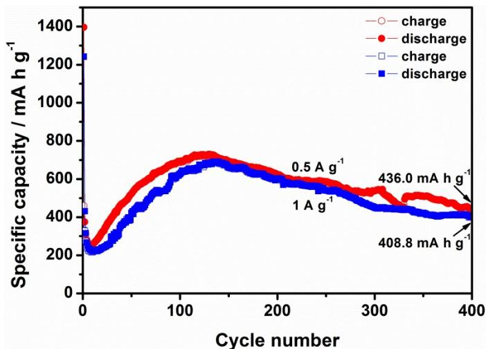
**Figure S7.** Cycling performance of Fe-BTC MOF at high current density ( $0.5 \text{ A g}^{-1}$  and  $1 \text{ A g}^{-1}$ ).
