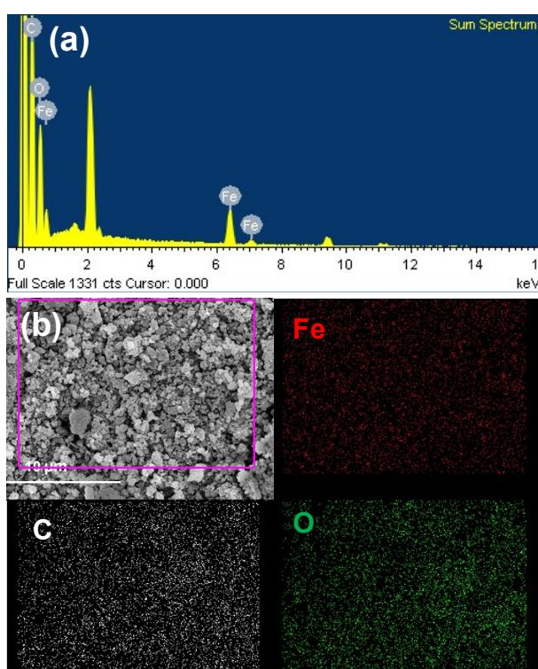
**Figure S4.** EDS spectra and EDS mapping images for a selected region of the synthetic Fe-BTC.
