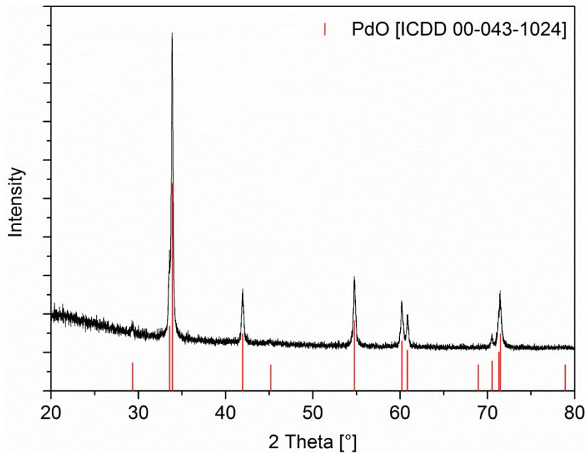
**SI 6.** XRPD pattern of the residue obtained by the TG of **8** under oxygen (gas flow, 20 sccm; heating rate  $10\text{ K min}^{-1}$ ).
