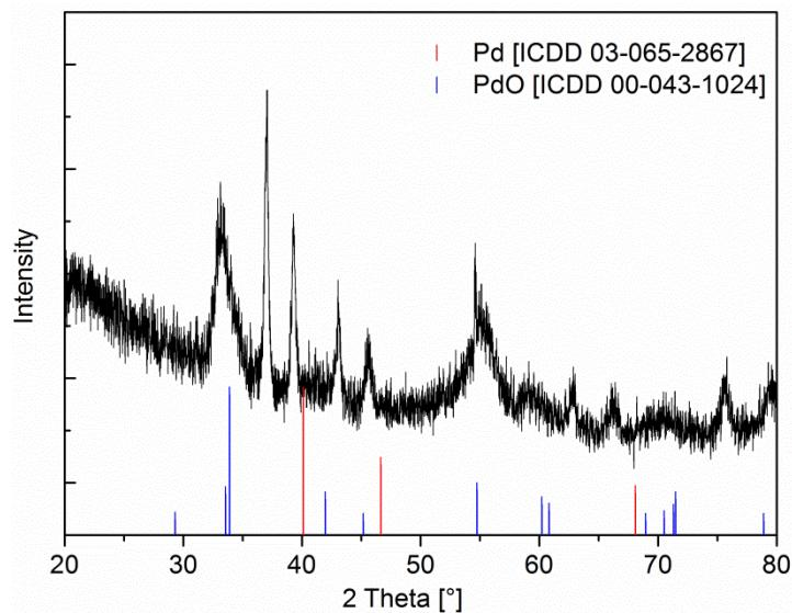
**SI 34.** XRPD pattern obtained from the layer formed by **14** CVD(O<sub>2</sub>).
