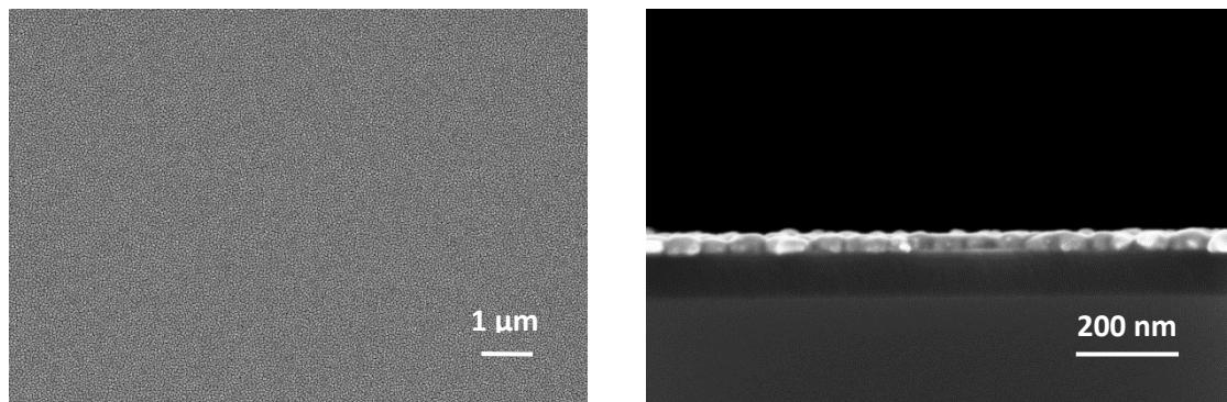
**SI 22.** Left: Layer obtained from the CVD( $N_2/H_2$ ) of **14**. Right: Cross-section image. Substrate temperature 350 °C, deposition time 15 min, nitrogen flow rate 40 sccm (carrier gas), forming gas 40 sccm, working pressure 0.8 mbar.
