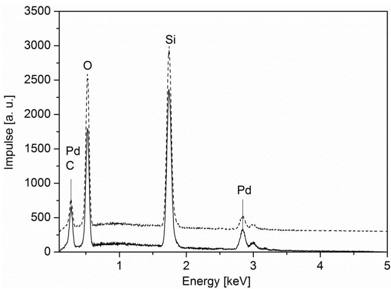
**SI 24.** EDX spectra of the film obtained from **12** by CVD( $O_2$ ) (dotted, oxygen flow rate 40 sccm, substrate temperature 380 °C) and CVD( $N_2/H_2$ ) (solid, forming gas flow rate 40 sccm, substrate temperature 350 °C) for comparison.
