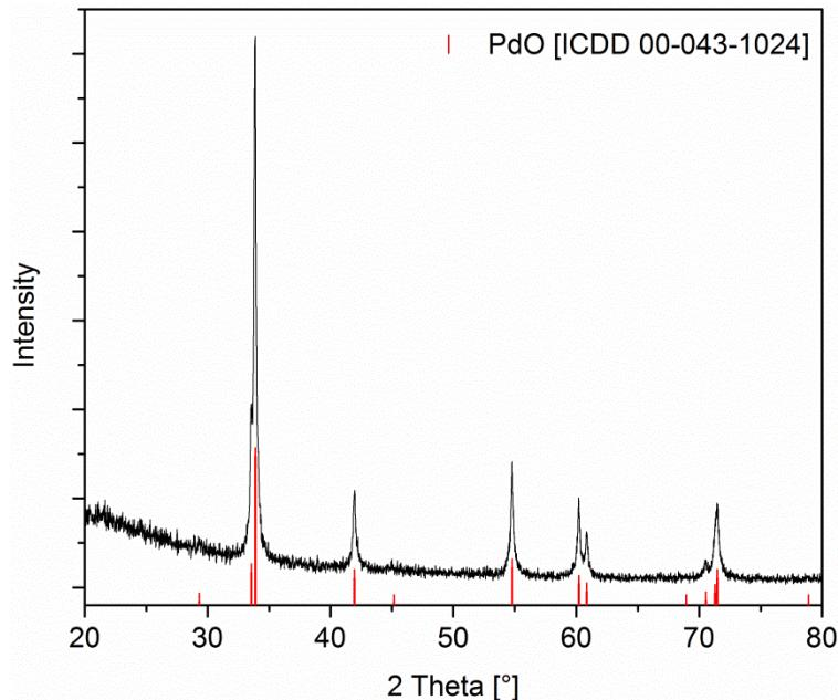
**SI 14.** XRPD pattern of the residue obtained by the TG of **14** under oxygen (gas flow, 20 sccm; heating rate  $10\text{ K min}^{-1}$ ).
