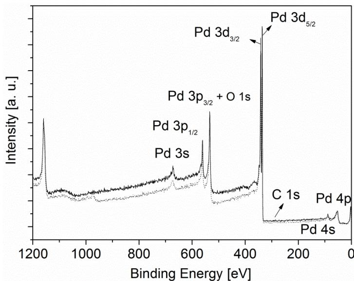
**SI 29.** *Ex-situ* XPS spectra of the film obtained from **13** by CVD(O<sub>2</sub>) (dotted, oxygen flow rate 40 sccm, substrate temperature 380 °C) and CVD(N<sub>2</sub>/H<sub>2</sub>) (solid, forming gas flow rate 40 sccm, substrate temperature 350 °C) for comparison.
