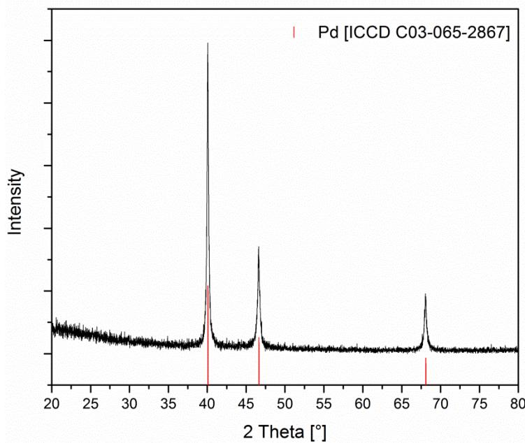
**SI 9.** XRPD pattern of the residue obtained by the TG of **12** under nitrogen (gas flow, 20 sccm; heating rate  $10\text{ K min}^{-1}$ ).
