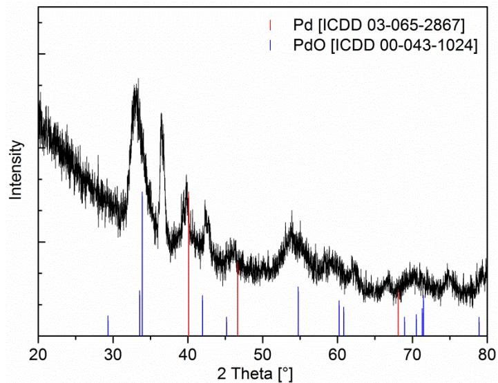
**SI 32.** XRPD pattern obtained from the layer formed by **11** CVD(O<sub>2</sub>).
