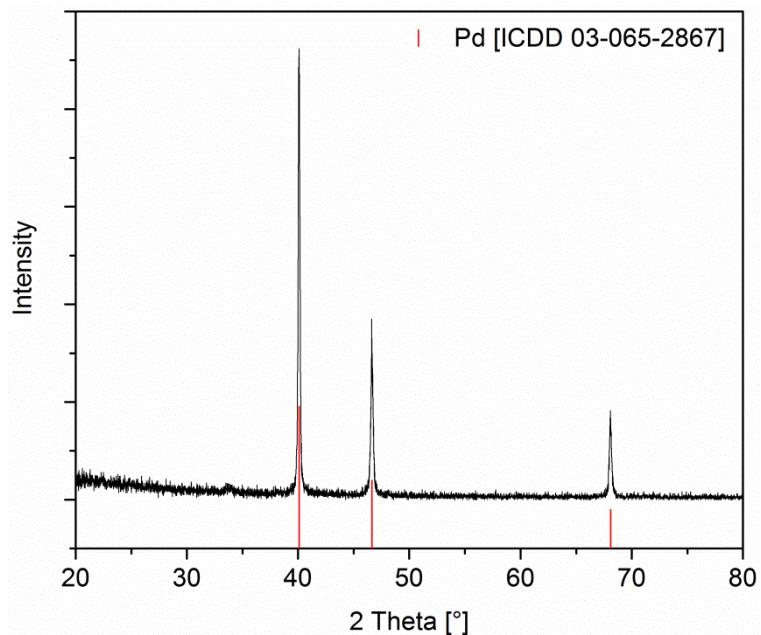
**SI 7.** XRPD pattern of the residue obtained by the TG of **11** under nitrogen (gas flow, 20 sccm; heating rate  $10\text{ K min}^{-1}$ ).
