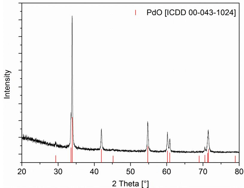
**SI 10.** XRPD pattern of the residue obtained by the TG of **12** under oxygen (gas flow, 20 sccm; heating rate  $10\text{ K min}^{-1}$ ).
