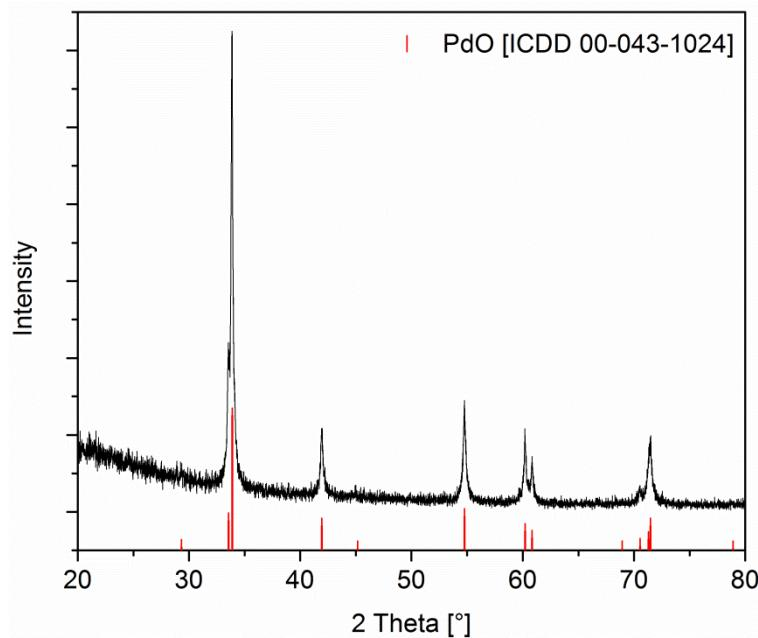
**SI 12.** XRPD pattern of the residue obtained by the TG of **13** under oxygen (gas flow, 20 sccm; heating rate 10 K min<sup>-1</sup>).
