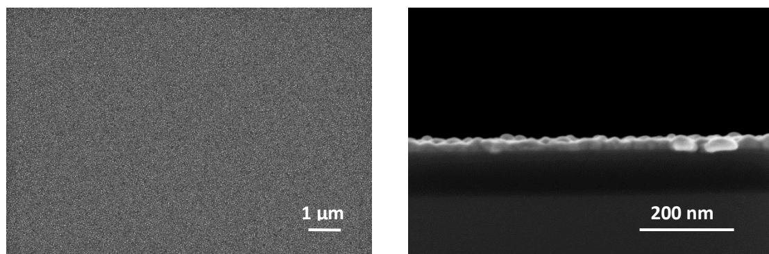
**SI 17.** Left: Layer obtained from the CVD( $O_2$ ) of **12**. Right: Cross-section image. Substrate temperature 380 °C, deposition time 15 min, nitrogen flow rate 40 sccm (carrier gas), oxygen flow rate 40 sccm, working pressure 0.8 mbar.
