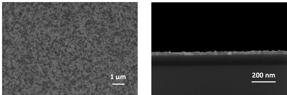
**SI 21.** Left: Layer obtained from the CVD( $O_2$ ) of **14**. Right: Cross-section image. Substrate temperature 380 °C, deposition time 15 min, nitrogen flow rate 40 sccm (carrier gas), oxygen flow rate 40 sccm, working pressure 0.8 mbar.
