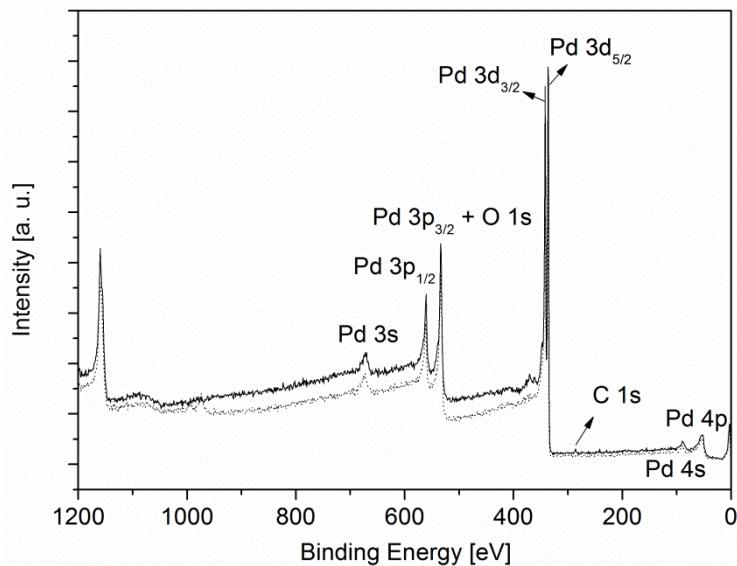
**SI 27.** *Ex-situ* XPS spectra of the film obtained from **11** by CVD(O<sub>2</sub>) (dotted, oxygen flow rate 40 sccm, substrate temperature 380 °C) and CVD(N<sub>2</sub>/H<sub>2</sub>) (solid, forming gas flow rate 40 sccm, substrate temperature 350 °C) for comparison.
