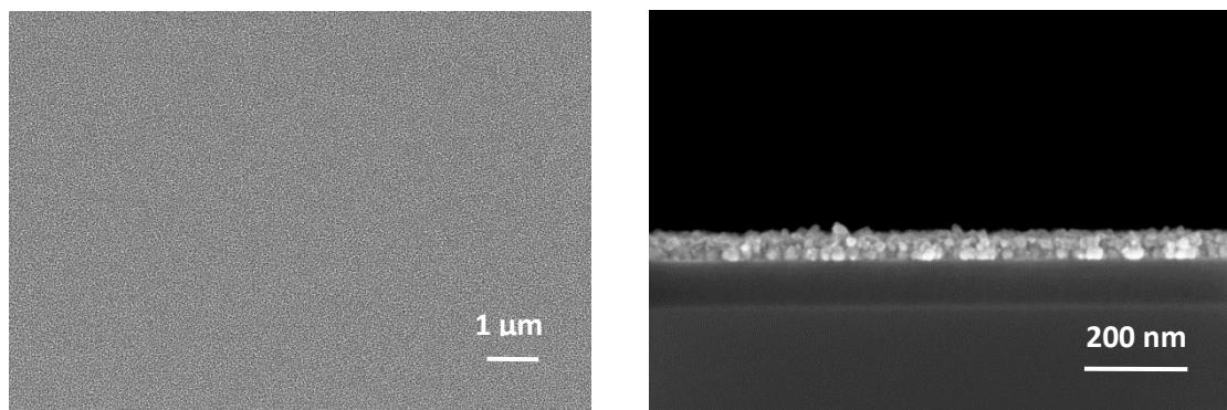
**SI 18.** Left: Layer obtained from the CVD( $\text{N}_2/\text{H}_2$ ) of **12**. Right: Cross-section image. Substrate temperature 350 °C, deposition time 15 min, nitrogen flow rate 40 sccm (carrier gas), forming gas 40 sccm, working pressure 0.8 mbar.
