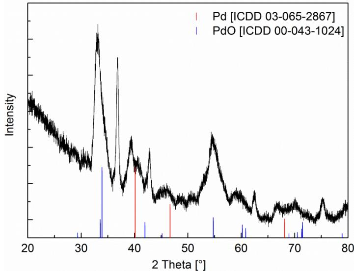
**SI 33.** XRPD pattern obtained from the layer formed by **12** CVD(O<sub>2</sub>).
