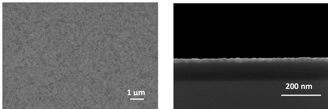
**SI 19.** Left: Layer obtained from the CVD( $\text{O}_2$ ) of **13**. Right: Cross-section image. Substrate temperature 380 °C, deposition time 15 min, nitrogen flow rate 40 sccm (carrier gas), oxygen flow rate 40 sccm, working pressure 0.8 mbar.
