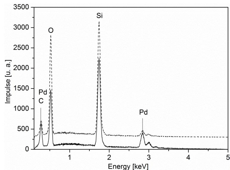
**SI 26.** EDX spectra of the film obtained from **14** by CVD(O<sub>2</sub>) (dotted, oxygen flow rate 40 sccm, substrate temperature 380 °C) and CVD(N<sub>2</sub>/H<sub>2</sub>) (solid, forming gas flow rate 40 sccm, substrate temperature 350 °C) for comparison.
