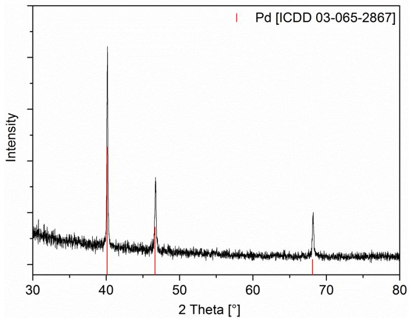
**SI 5.** XRPD pattern of the residue obtained by the TG of **8** under nitrogen (gas flow, 20 sccm; heating rate  $10\text{ K min}^{-1}$ ).
