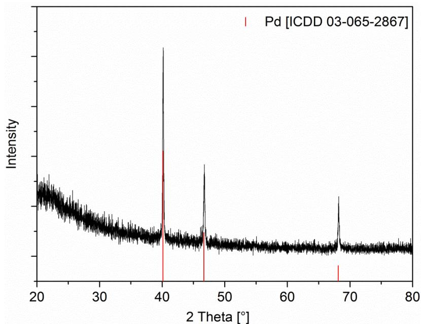
**SI 3.** XRPD pattern of the residue obtained by the TG of **7** under nitrogen (gas flow, 20 sccm; heating rate  $10\text{ K min}^{-1}$ ).
