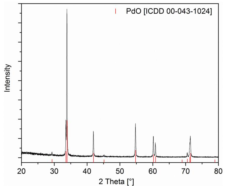
**SI 8.** XRPD pattern of the residue obtained by the TG of **11** under oxygen (gas flow, 20 sccm; heating rate  $10\text{ K min}^{-1}$ ).
