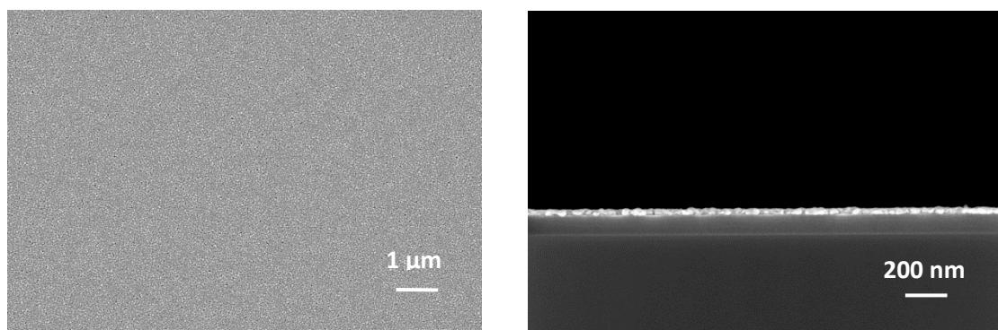
**SI 20.** Left: Layer obtained from the CVD( $\text{N}_2/\text{H}_2$ ) of **13**. Right: Cross-section image. Substrate temperature 350 °C, deposition time 15 min, nitrogen flow rate 40 sccm (carrier gas), forming gas 40 sccm, working pressure 0.8 mbar.
