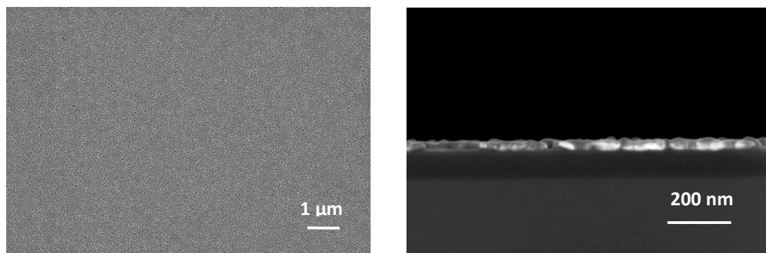
**SI 16.** Left: Layer obtained from the CVD( $N_2/H_2$ ) of **11**. Right: Cross-section image. Substrate temperature 350 °C, deposition time 15 min, nitrogen flow rate 40 sccm (carrier gas), forming gas 40 sccm, working pressure 0.8 mbar.
