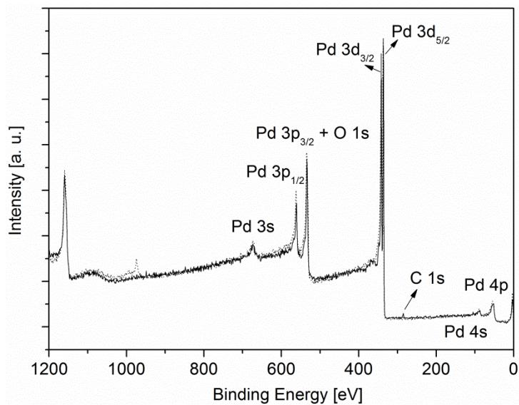
**SI 30.** *Ex-situ* XPS spectra of the film obtained from **14** by CVD(O<sub>2</sub>) (dotted, oxygen flow rate 40 sccm, substrate temperature 380 °C) and CVD(N<sub>2</sub>/H<sub>2</sub>) (solid, forming gas flow rate 40 sccm, substrate temperature 350 °C) for comparison.
