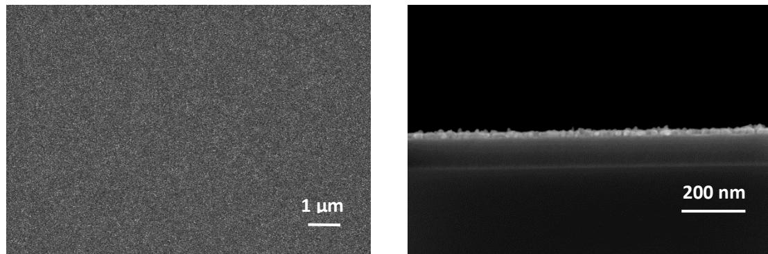
**SI 15.** Left: Layer obtained from the CVD( $O_2$ ) of **11**. Right: Cross-section image. Substrate temperature 380 °C, deposition time 15 min, nitrogen flow rate 40 sccm (carrier gas), oxygen flow rate 40 sccm, working pressure 0.8 mbar.
