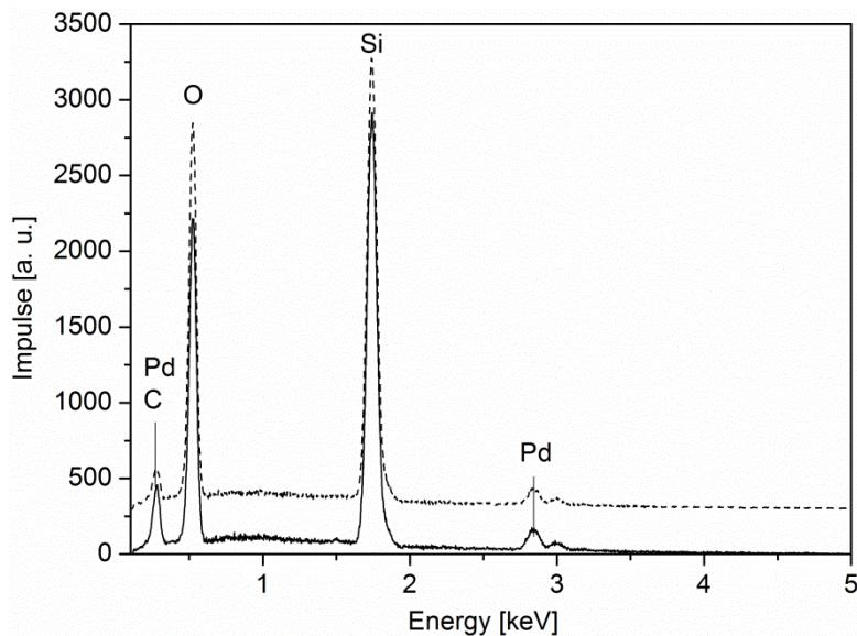
**SI 23.** EDX spectra of the film obtained from **11** by CVD( $O_2$ ) (dotted, oxygen flow rate 40 sccm, substrate temperature 380 °C) and CVD( $N_2/H_2$ ) (solid, forming gas flow rate 40 sccm, substrate temperature 350 °C) for comparison.
