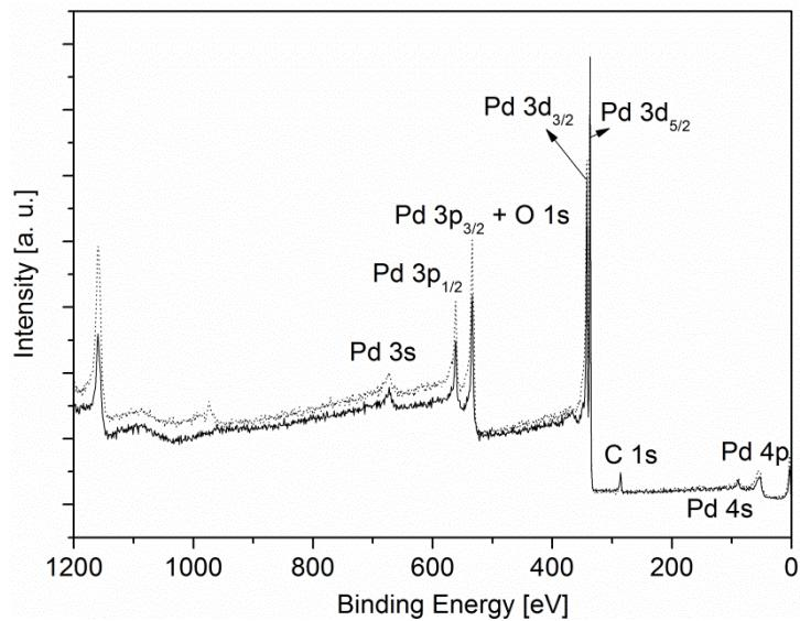
**SI 28.** *Ex-situ* XPS spectra of the film obtained from **12** by CVD(O<sub>2</sub>) (dotted, oxygen flow rate 40 sccm, substrate temperature 380 °C) and CVD(N<sub>2</sub>/H<sub>2</sub>) (solid, forming gas flow rate 40 sccm, substrate temperature 350 °C) for comparison.
