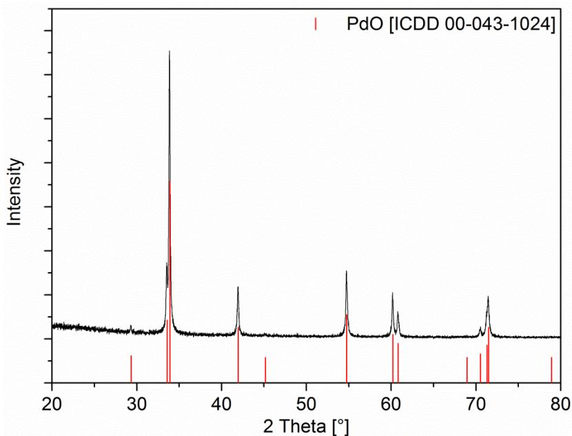
**SI 4.** XRPD pattern of the residue obtained by the TG of **7** under oxygen (gas flow, 20 sccm; heating rate  $10\text{ K min}^{-1}$ ).
