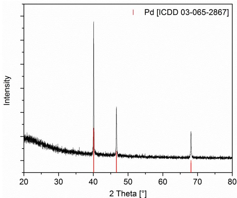
**SI 13.** XRPD pattern of the residue obtained by the TG of **14** under nitrogen (gas flow, 20 sccm; heating rate  $10\text{ K min}^{-1}$ ).
