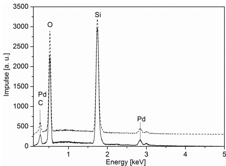
**SI 25.** EDX spectra of the film obtained from **13** by CVD(O<sub>2</sub>) (dotted, oxygen flow rate 40 sccm, substrate temperature 380 °C) and CVD(N<sub>2</sub>/H<sub>2</sub>) (solid, forming gas flow rate 40 sccm, substrate temperature 350 °C) for comparison.
