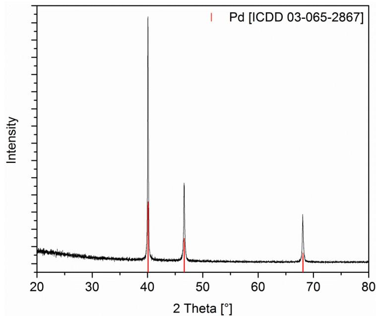
**SI 11.** XRPD pattern of the residue obtained by the TG of **13** under nitrogen (gas flow, 20 sccm; heating rate 10 K min<sup>-1</sup>).
