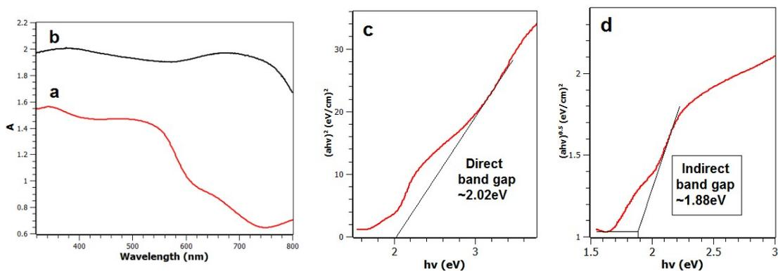
Fig. S2. Solid state UV-visible spectroscopy of catalysts showing (a) Fe<sub>2</sub>O<sub>3</sub>; (b) commercial Co<sub>3</sub>O<sub>4</sub>; (c) Tauc plot showing direct band gap of ~2.02eV of the Fe<sub>2</sub>O<sub>3</sub> catalyst; (d) Tauc plot showing visible light indirect band gap of ~1.88eV of the Fe<sub>2</sub>O<sub>3</sub> catalyst.
