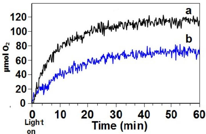
Fig.S5. Graph of released O<sub>2</sub> (µmol) against time for photocatalyzed water oxidation reactions with a Co<sub>3</sub>O<sub>4</sub> catalyst using (a) repeating 50s cycle light source,  $\bar{x} = 3.3 \text{ mWcm}^{-2}$ ; (b) blue light ( $\lambda_{\text{max}} 455 \text{ nm}$ ) @  $5 \text{ mWcm}^{-2}$ .
