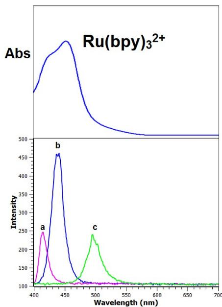
Fig. S3. Graph of measured relative intensity and wavelengths of led emissions used as combined [Ru(bpy)<sub>3</sub>]<sup>2+</sup> saturation light source in photocatalytic water oxidation reactions showing (a) 410; (b) 450 and (c) 500 nm maximum wavelengths. The visible light absorption spectrum of [Ru(bpy)<sub>3</sub>]<sup>2+</sup> is shown for comparison.
