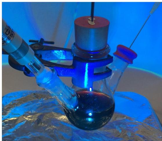
Image of reaction flask containing optical O<sub>2</sub> sensor and stirred reaction mixture with pH and temperature probe.
