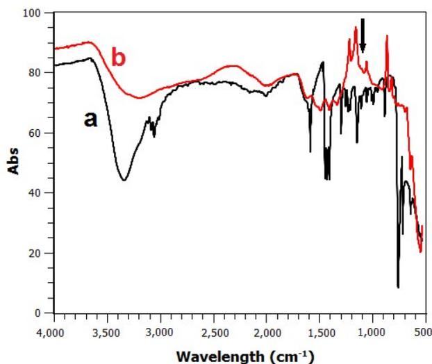
Fig. S6. Graph of FT-IR of (a)  $[\text{Ru}(\text{bpy})_3]\text{Cl}_2 \cdot 6\text{H}_2\text{O}$ ; (b) low solubility decomposition material deposited during a photocatalytic water oxidation onto glass flask surface. The breakdown material was composed of bipyridine together with hydroxylated- $\text{Ru}(\text{bpy})_2^{2+}$  derivatives as indicated by a prominent band at  $\sim 1120\text{cm}^{-1}$  (arrowed) which corresponds to a C-O(str).[2]
