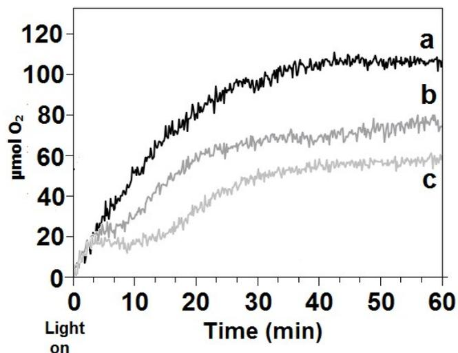
Fig. S4. Graph of released O<sub>2</sub> (µmol) against time for photocatalyzed water oxidation reactions with a  $\alpha$ -Fe<sub>2</sub>O<sub>3</sub> catalyst, reactions illuminated for 60min were conducted using a light source with a repeating wavelength/ intensity cycle of duration (a) 50s; (b) 25s; (c) 100s.
