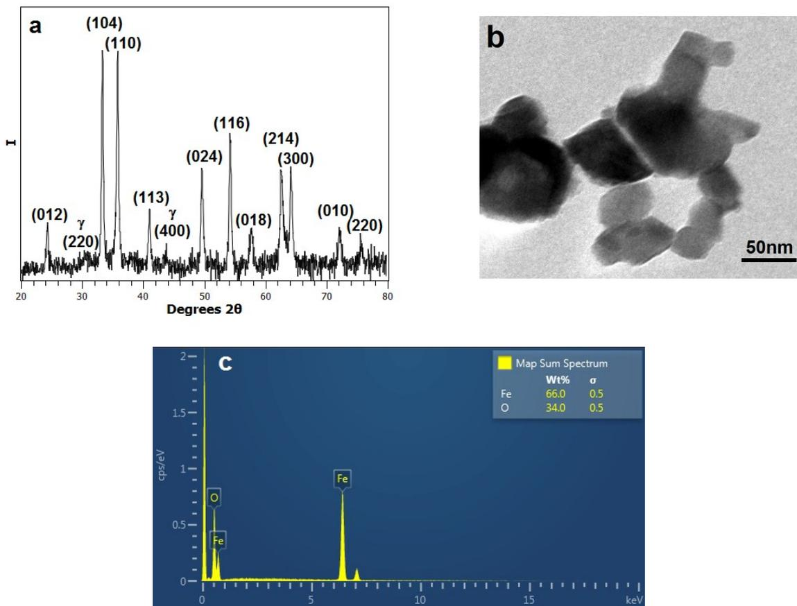
Fig.S1.(a) Powder XRD of  $\alpha$ -Fe<sub>2</sub>O<sub>3</sub> (JCPDS 013-0534, hematite) with trace level of  $\gamma$ -Fe<sub>2</sub>O<sub>3</sub> (JCPDS 024-081, maghemite) prepared by calcination with xyloglucan used as a sacrificial size limiting biopolymer; (b) TEM image of the  $\alpha$ -Fe<sub>2</sub>O<sub>3</sub> nanoparticles; (c) EDX analysis of the Fe<sub>2</sub>O<sub>3</sub> catalyst showing presence of iron and oxygen only.
