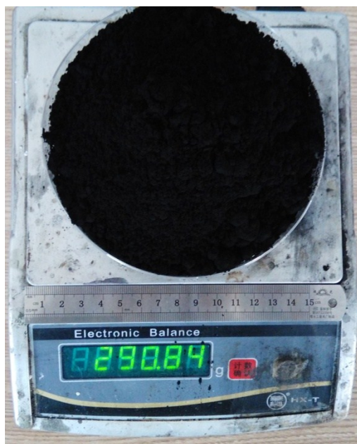
Fig. S1 Digital photograph of as-prepared full concentration gradient precursor \text{Ni}_{0.6}\text{Co}_{0.15}\text{Mn}_{0.25}(\text{OH})_2 .
