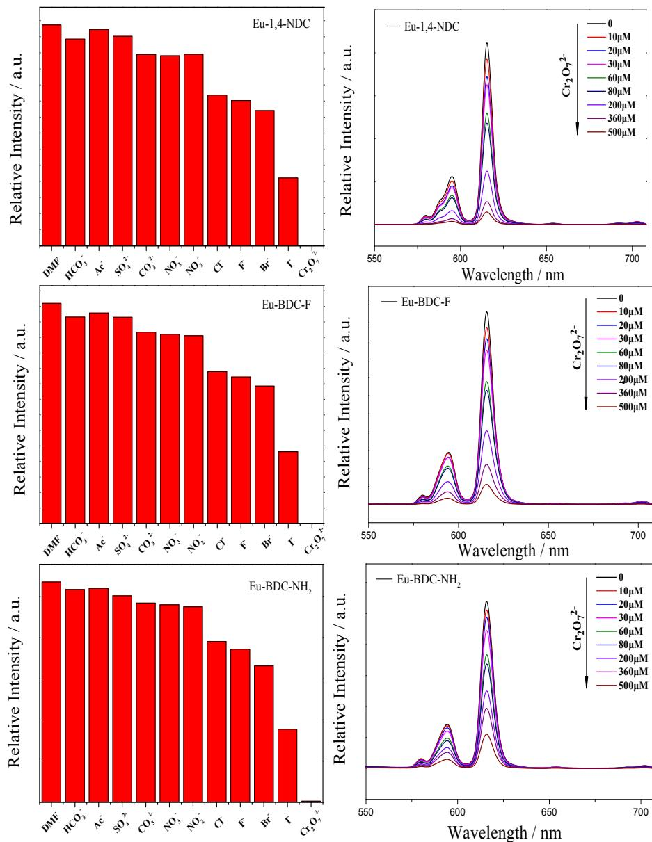
**Fig. S5** The PL intensities of Eu-MOFs toward with various anions and in various concentrations of Cr<sub>2</sub>O<sub>7</sub><sup>2-</sup> solution.
