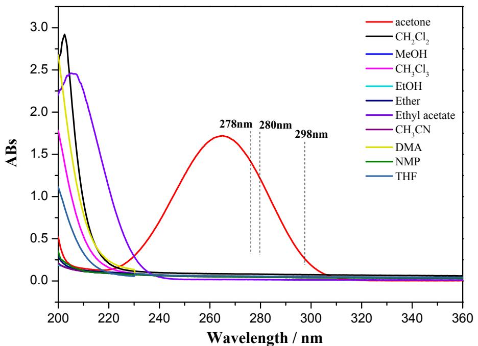
**Fig. S8** Liquid UV-vis absorption spectra of different solvents.
