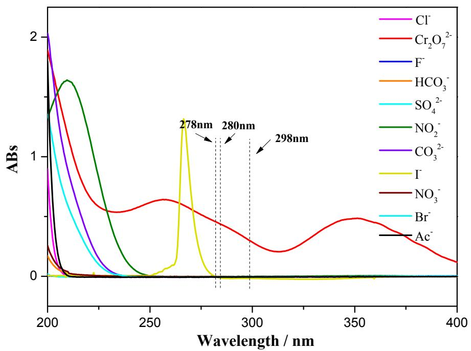
**Fig. S6** Liqiud UV-vis absorption spectra of different anions.
